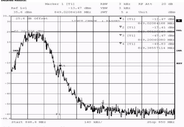
band edge compliance measurement Comment A: CS020, GSM850, band edge compliance, channel 251 (848.8MHz)
