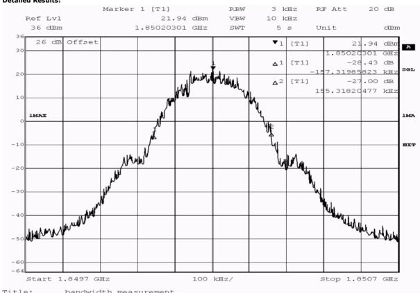
bandwidth measurement CSOZO, GSM1900, 26dB bandwidth, channel 512 (1850.2MHz)
