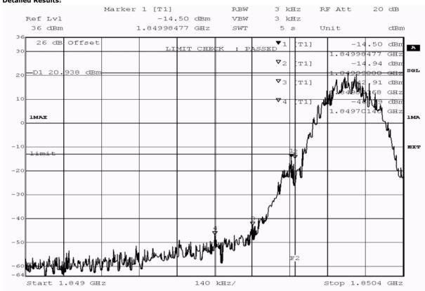
band edge compliance measurement Comment A: CS020, GSM1900, band edge compliance, channel 512 (1850.2MHz)
