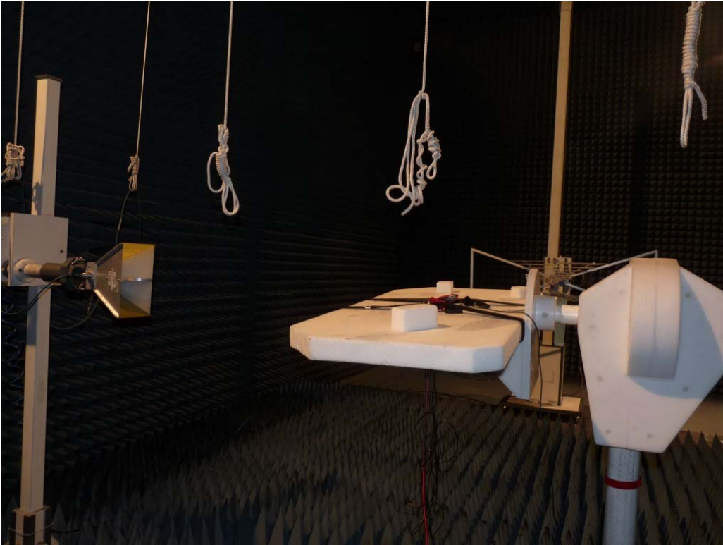
Photo 2: Test setup for radiated measurements (Enclosure, fully-anechoic chamber, 1-18 GHz intentional radiator §15 / 30 MHz – 10/20 GHz §22/24/27)
