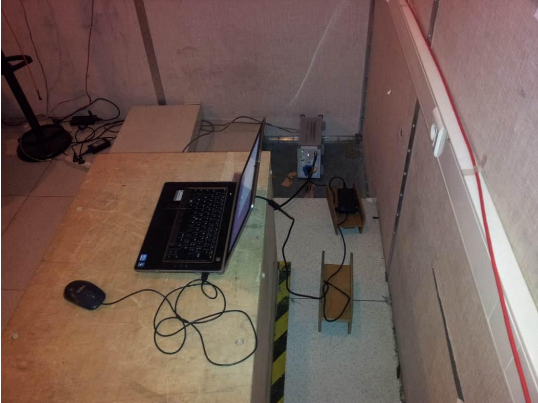
Conducted emission measurements
