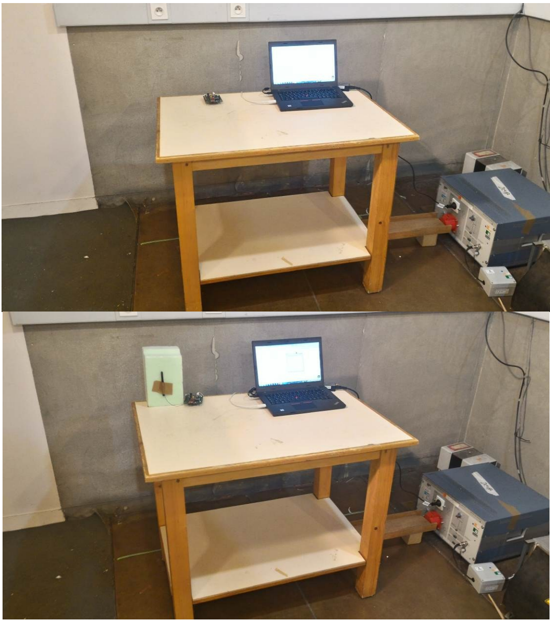
Photograph for AC Power Line Conducted Emissions (Rear view)
