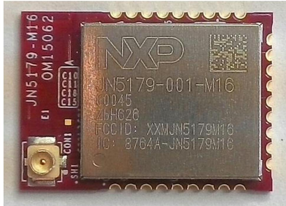
Label location is on top of the module. It's laser marked on the metal shield
