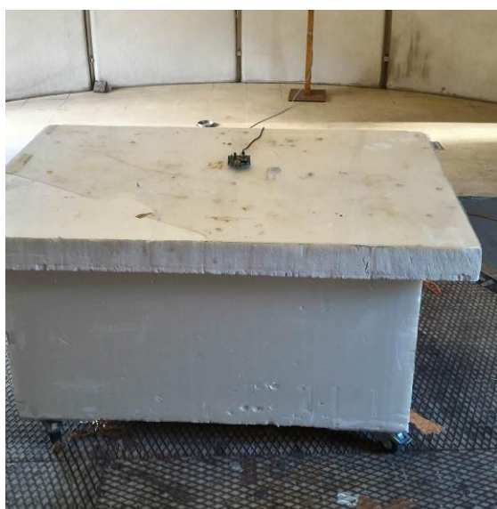
Radiated emissions measurements setup below 1.5GHz (3V & 6V)
