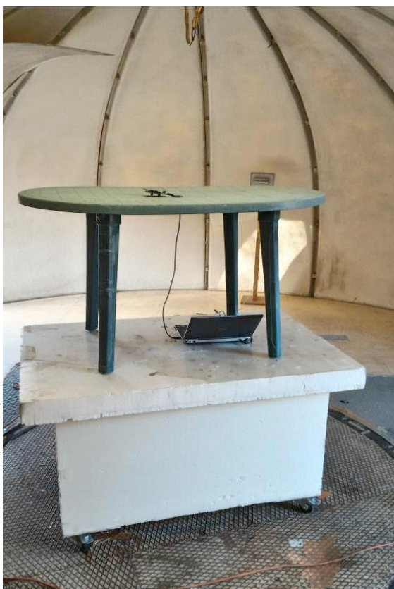
Radiated emissions measurements setup above 1.5GHz (3V & 6V)
