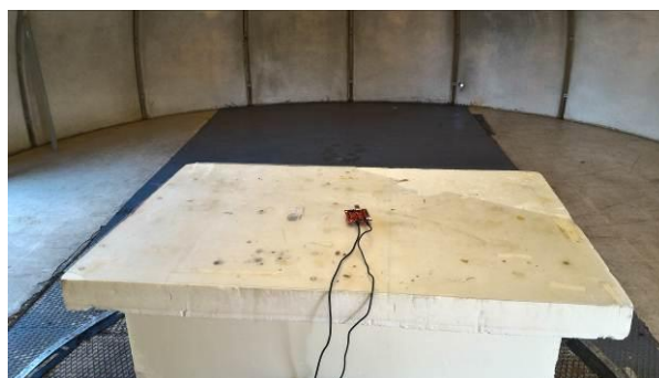
Radiated emissions measurements setup below 1.5GHz (3V & 6V)
