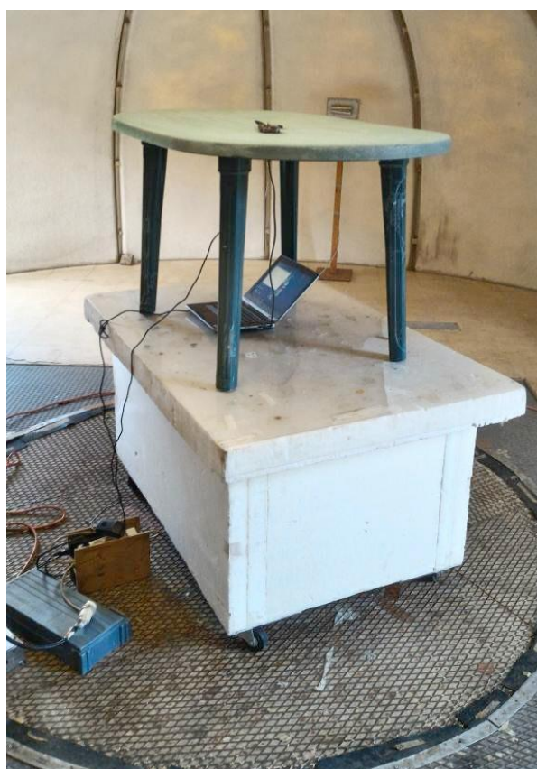
Radiated emissions measurements setup above 1.5GHz (3V & 6V)
