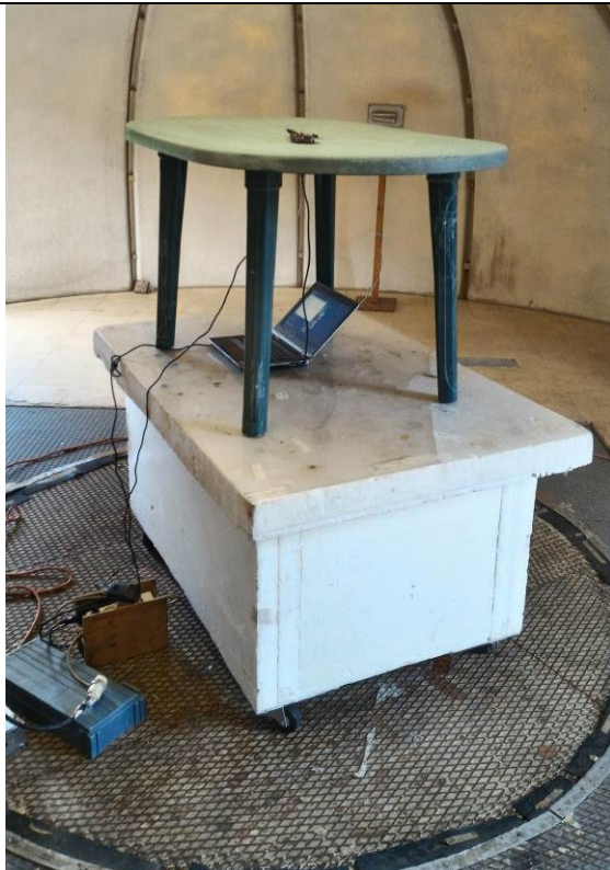
Photograph for Unwanted Emissions into Restricted Frequency Bands (JN5179-001-M00 -power supply 6V)
