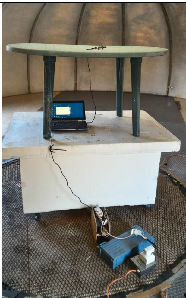
Photograph for Unwanted Emissions into Restricted Frequency Bands (JN5179-001-M00 -power supply 3V)
