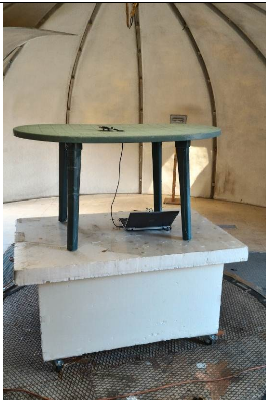
Photograph for Unwanted Emissions into Restricted Frequency Bands (JN5179-001-M00 -power supply 3V)
