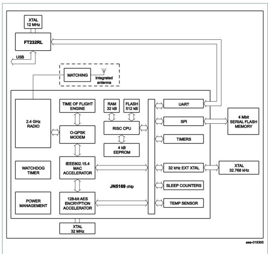
Fig 3. JN5169-001-U00-2 USB dongle hardware blocks
