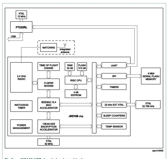
Fig 3. JN5169 USB dongle hardware blocks
