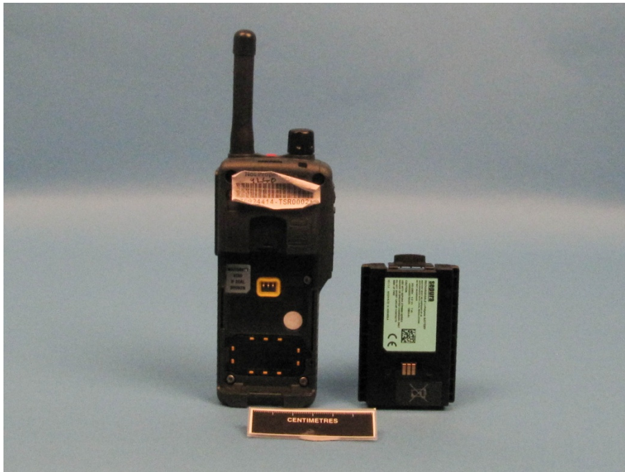
STP9240 Battery Removed
