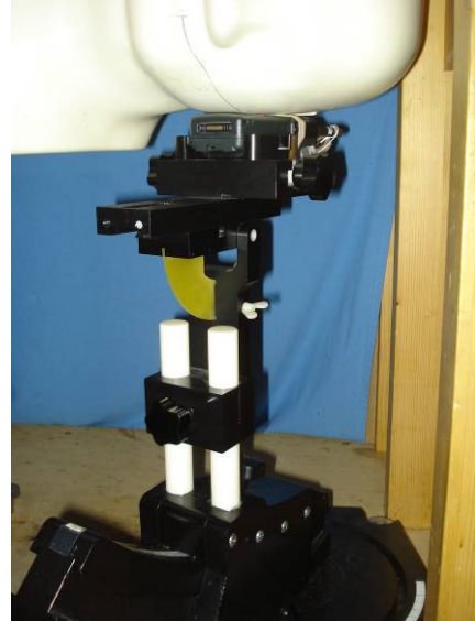
Held-to-Ear Test Setup – STP9240, -00662 Antenna, Left ear touch position
