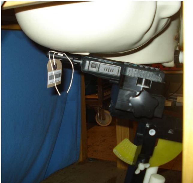
Held-to-Ear Test Setup – STP9040, -00663 Antenna, Right ear tilt position
