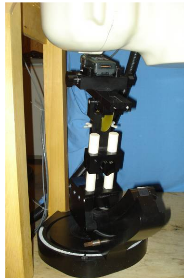
Held-to-Ear Test Setup – STP9240, -00662 Antenna, Right ear tilt position
