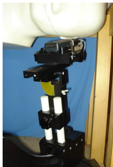
Held-to-Ear Test Setup – STP9040, -00663 Antenna, Left ear tilt position
