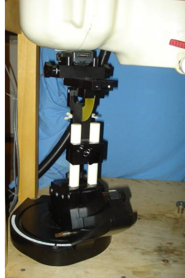
Held-to-Ear Test Setup – STP9040, -00663 Antenna, Right ear touch position
