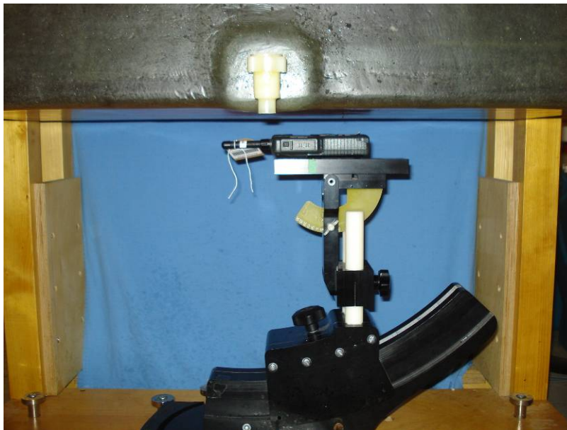
Face-Held Test Setup – STP9240, -00662 Antenna, -00634 Battery
