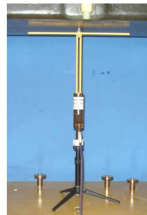
SPEAG 450 MHz Validation Dipole Setup
