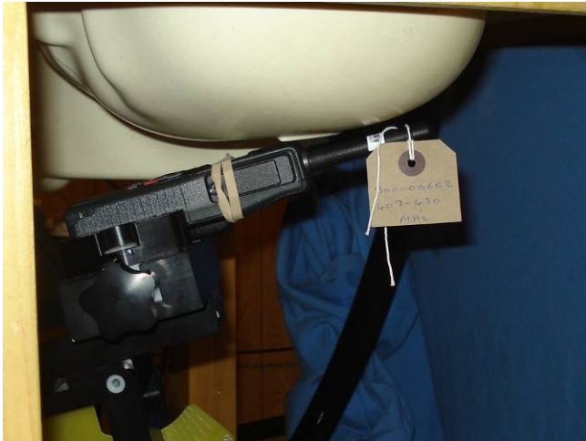
Held-to-Ear Test Setup – STP9240, -00662 Antenna, Left ear tilt position
