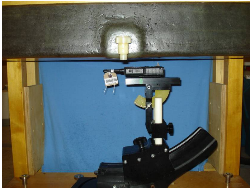
Face-Held Test Setup – STP9240, -00662 Antenna, -00635 Battery
