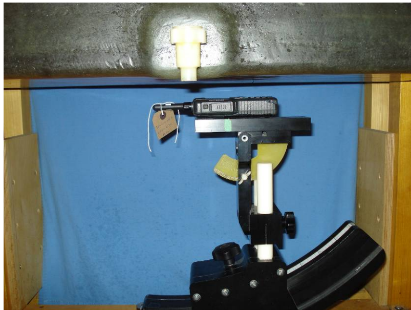
Face-Held Test Setup – STP9040, -00663 Antenna, -00634 Battery
