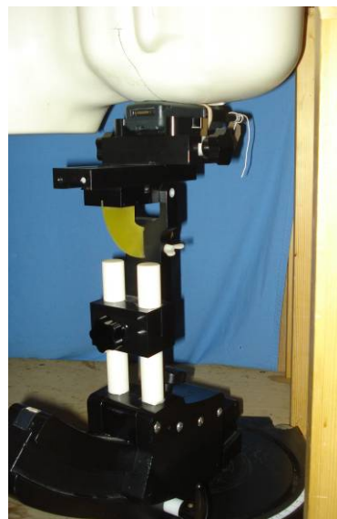
Held-to-Ear Test Setup STP9040, -00663 Antenna, Left ear touch position
