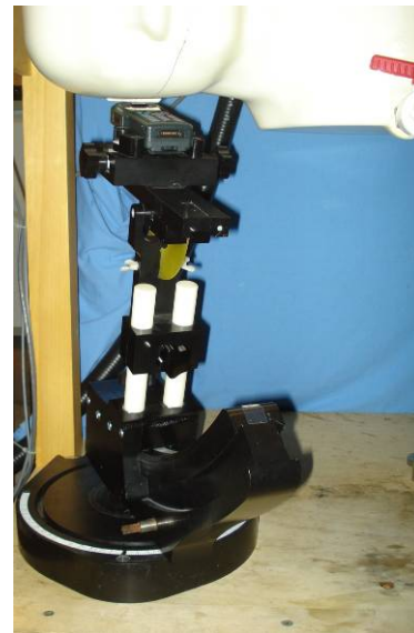
Held-to-Ear Test Setup – STP9040, -00663 Antenna, Right ear tilt position
