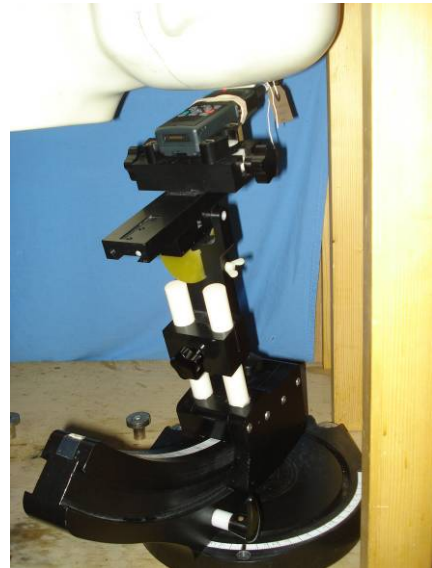
Held-to-Ear Test Setup – STP9240, -00662 Antenna, Left ear tilt position
