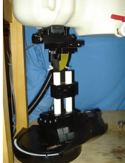
Held-to-Ear Test Setup – STP9240, -00662 Antenna, Right ear touch position
