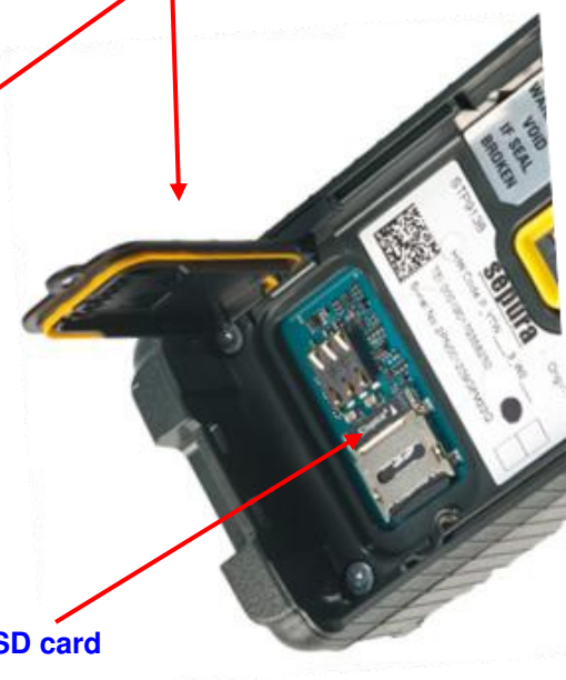
SIM Card holder/Micro SD card cover (open)
