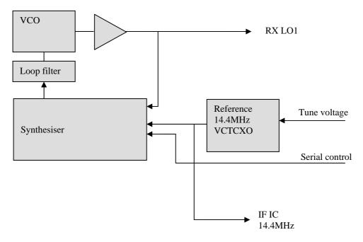
The local oscillator signal (RX LO)1 is at carrier frequency plus IF frequency A 14.4MHz reference signal (fed to a synthesiser on-board the receiver IF IC) enables conversion of the IF signal to base-band I and Q quadrature components.
