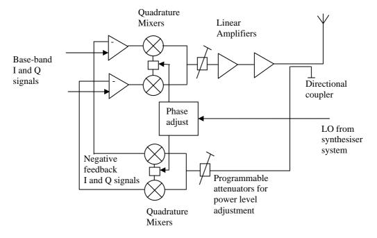
The implementation of the Cartesian loop, involves the use of an integrated Cartesian loop IC operating at the final carrier frequency. The injection signal from the frequency synthesiser is at 2 times the carrier frequency. This is illustrated in the diagram below.
