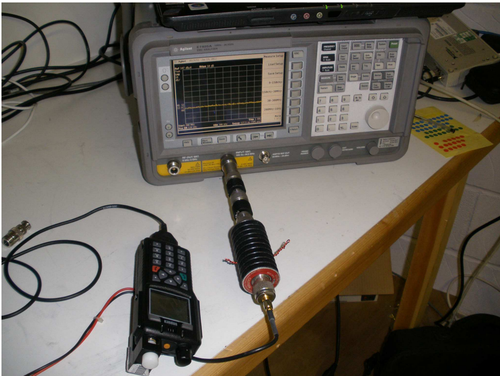
Photograph 2 STP8040: Connected to Agilent Analyser
