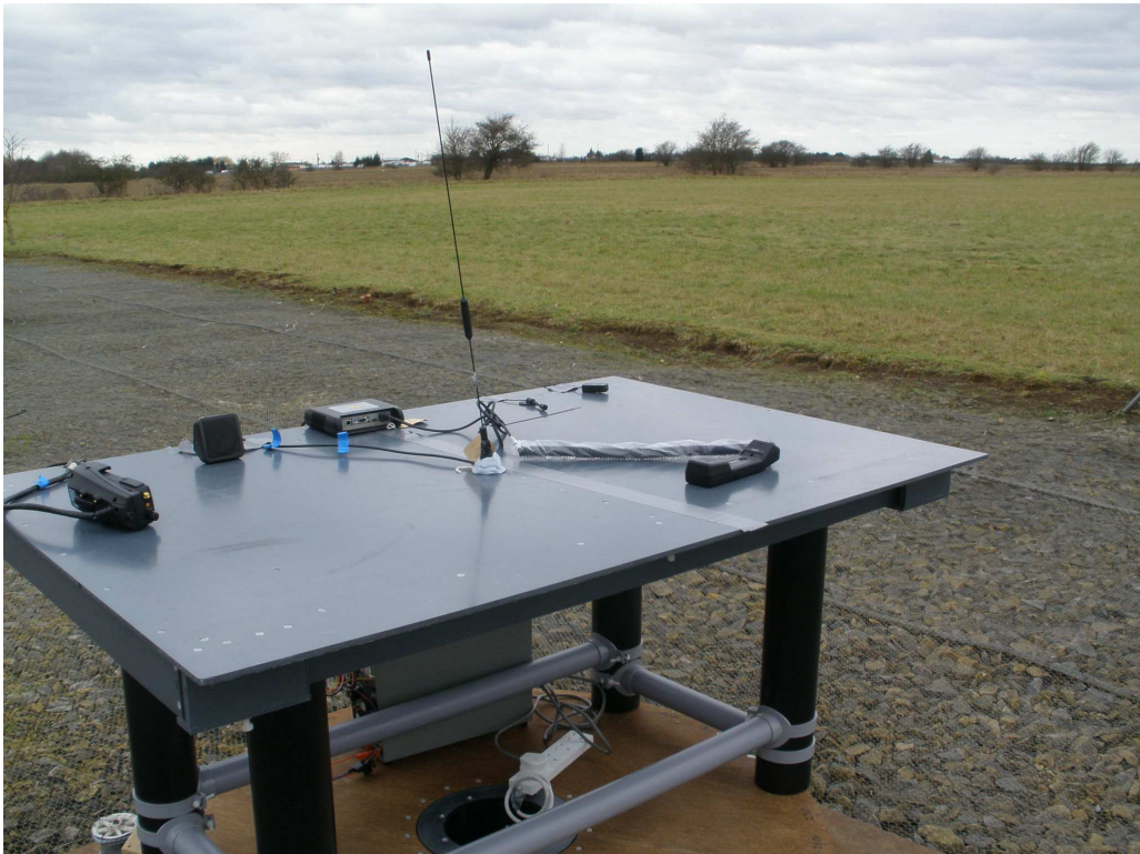
Photograph 3 Car Kit: Radiated Emissions - Front
