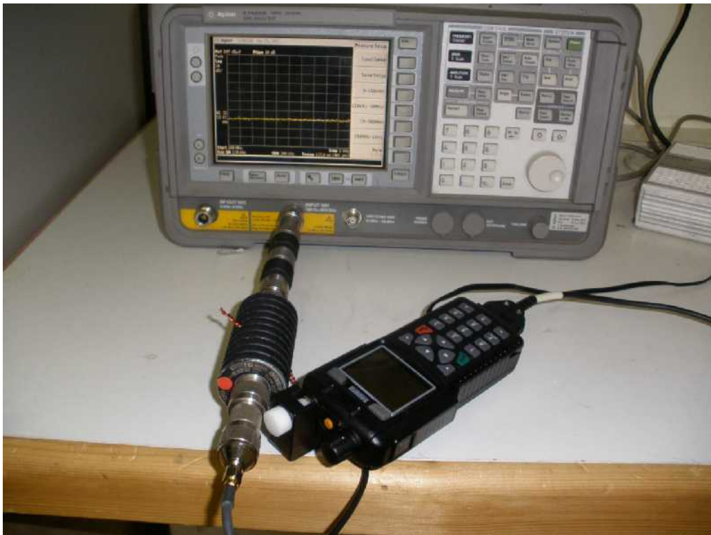
Photograph 1 STP8080: Connected to Agilent Analyser
