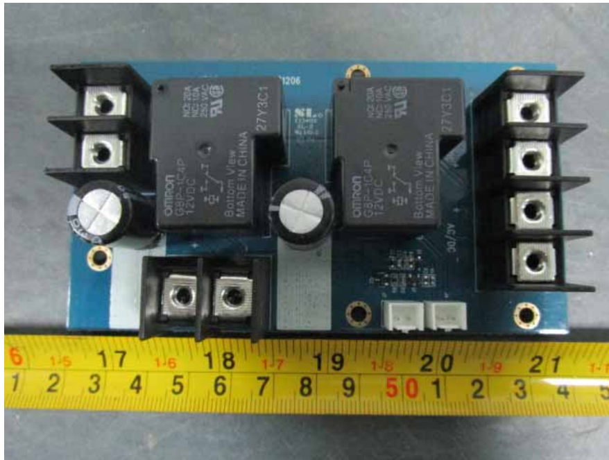
EUT- Power Controller Board Top View
