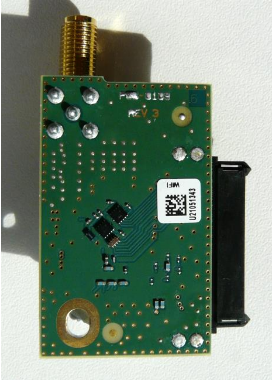
Figure 12. BT/Wi-Fi Board Bottom
