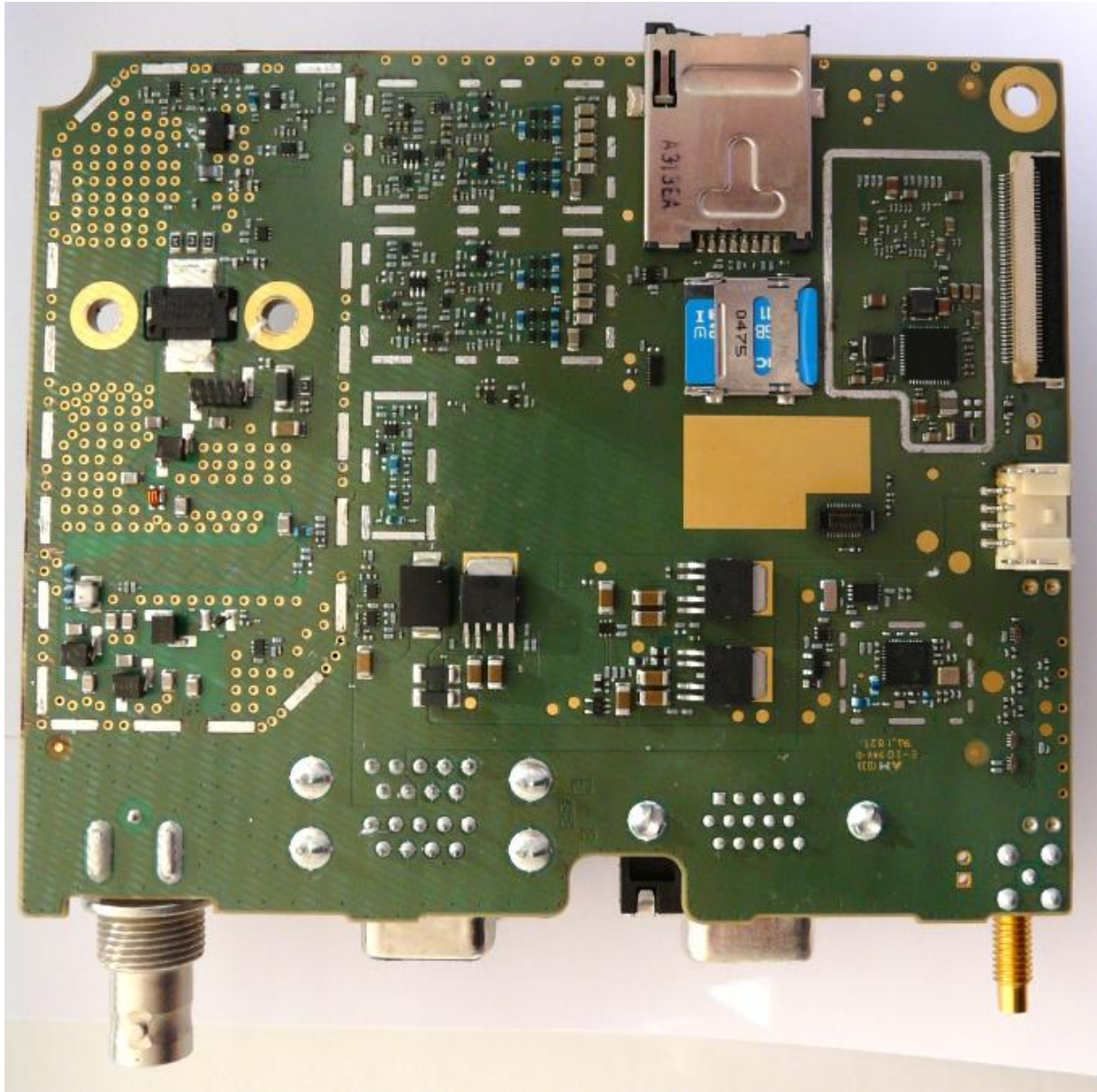
Figure 2. Main Board Bottom with cans removed
