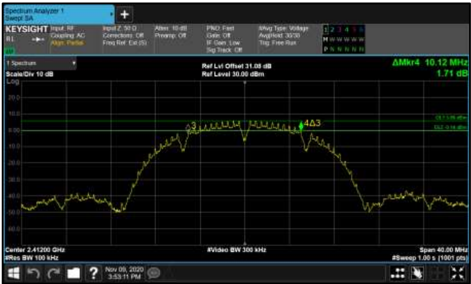
Figure 10 - (A) 2412 MHz (CH1) 6 dB Bandwidth
