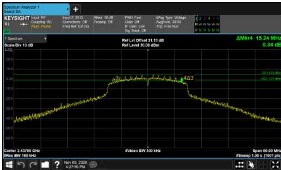
Figure 24 - (A) 2437 MHz (CH6) 6 dB Bandwidth
