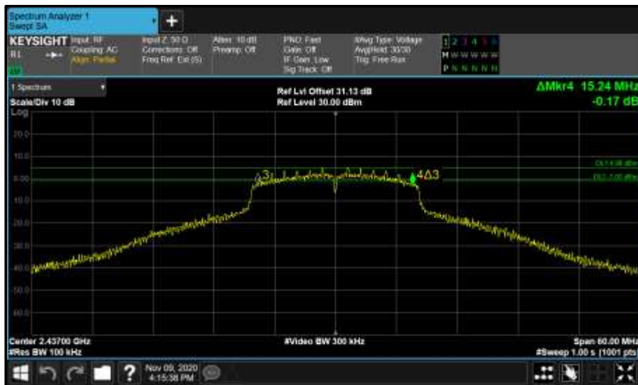
Figure 18 - (A) 2437 MHz (CH6) 6 dB Bandwidth
