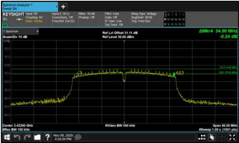
Figure 28 - (A) 2422 MHz (CH3) 6 dB Bandwidth
