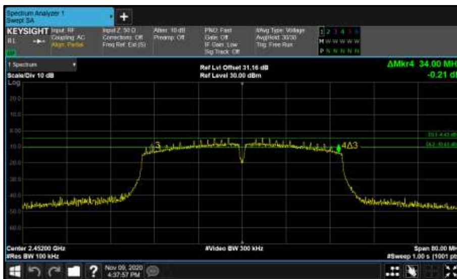
Figure 32 - (A) 2452 MHz (CH9) 6 dB Bandwidth
