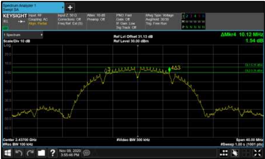
Figure 12 - (A) 2437 MHz (CH6) 6 dB Bandwidth
