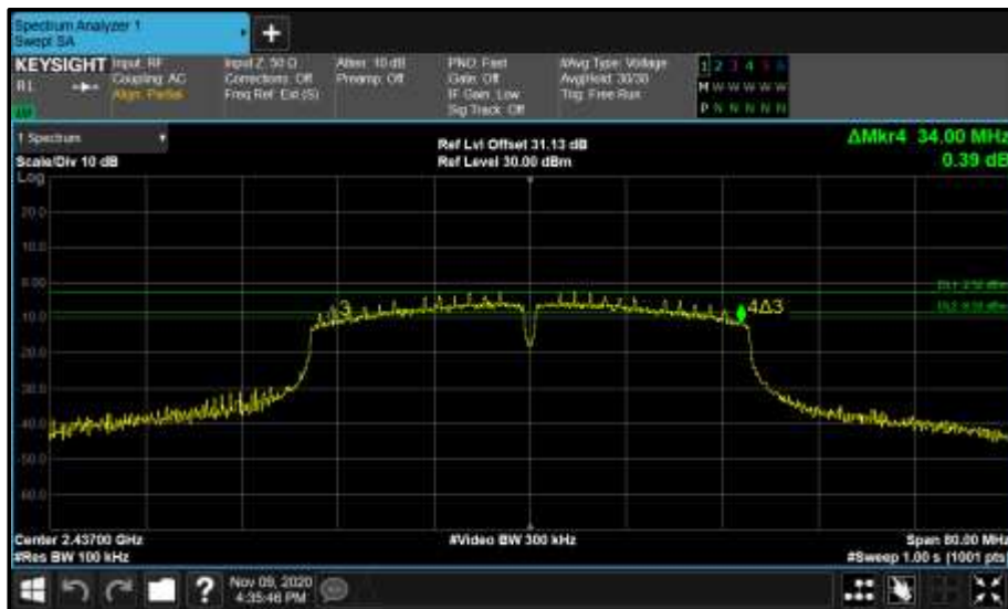
Figure 30 - (A) 2437 MHz (CH6) 6 dB Bandwidth
