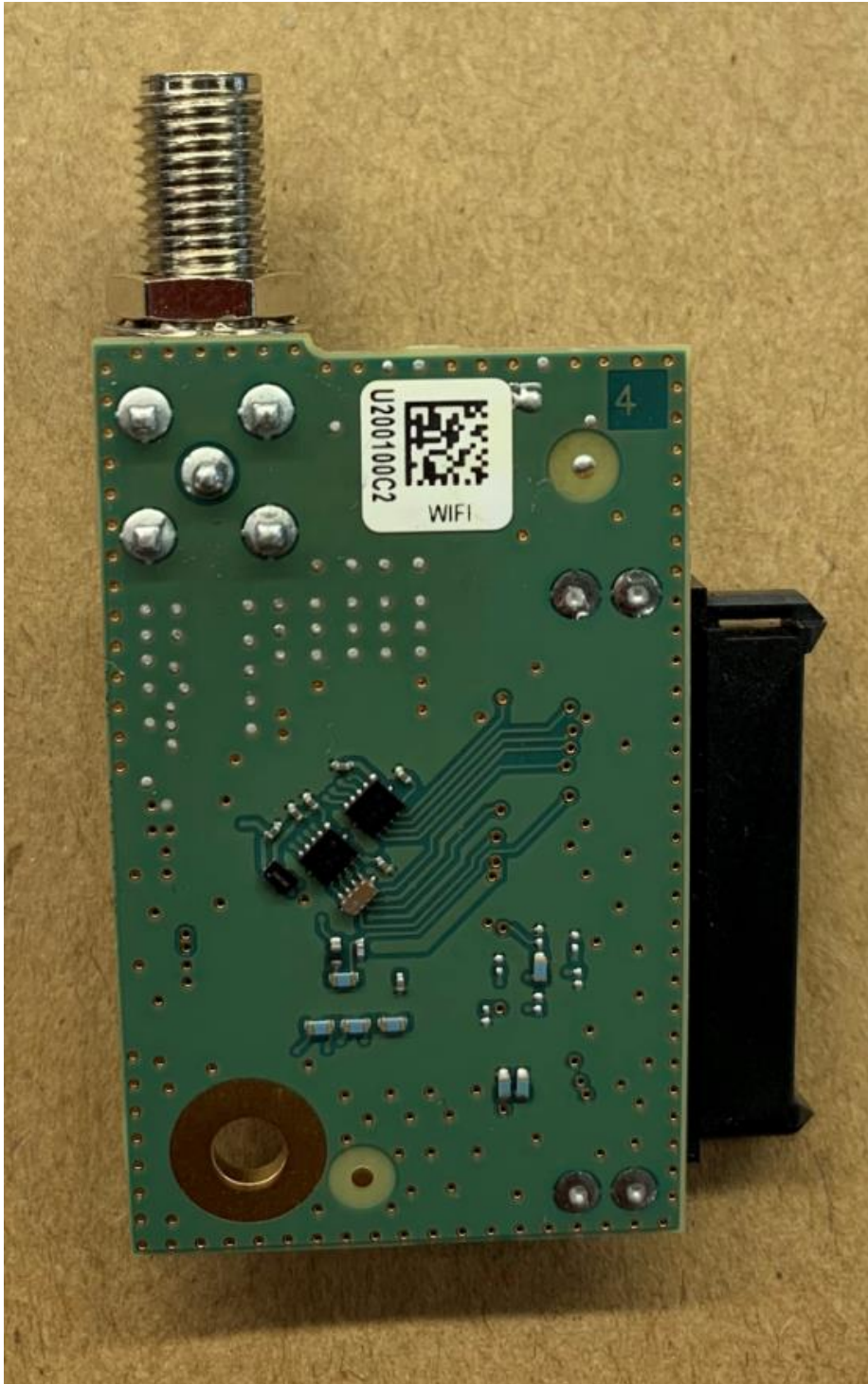
Figure 12. SCG2229 / XX6SCG2229 / 8739A-SCG2229 BT/Wi-Fi Board Bottom
