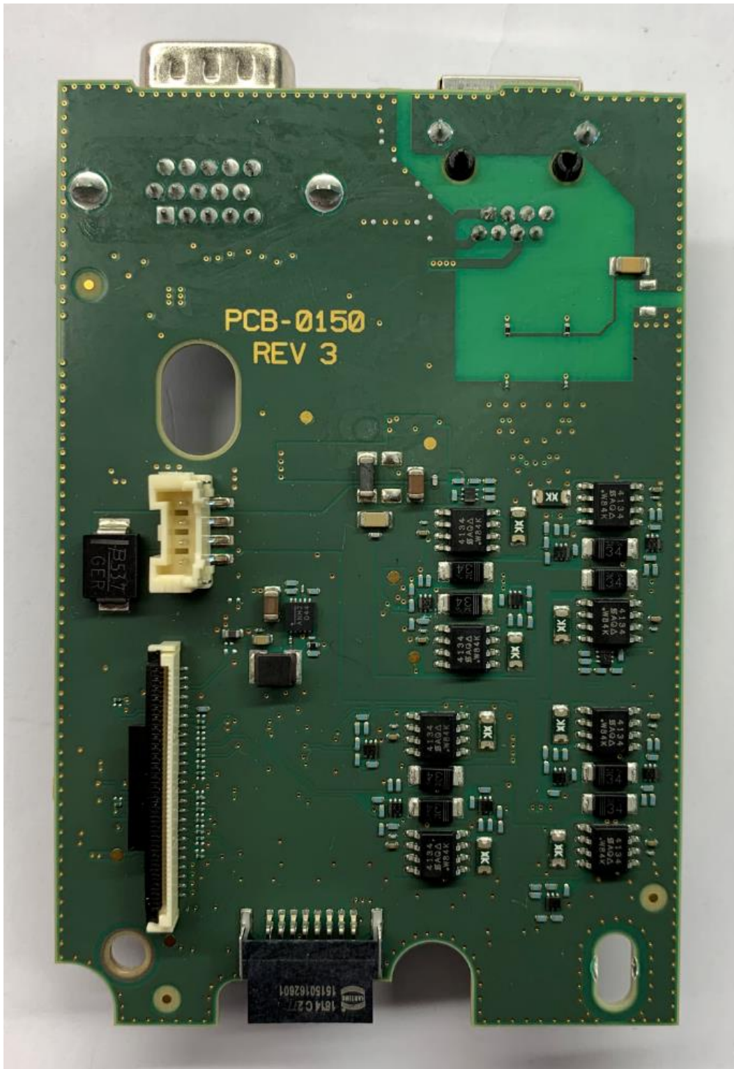
Figure 7. SCG2229 / XX6SCG2229 / 8739A-SCG2229 Expansion Board Bottom
