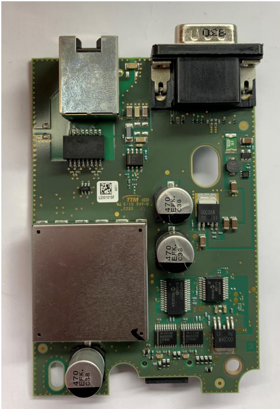
Figure 5. SCG2229 / XX6SCG2229 / 8739A-SCG2229 Expansion Board Top
