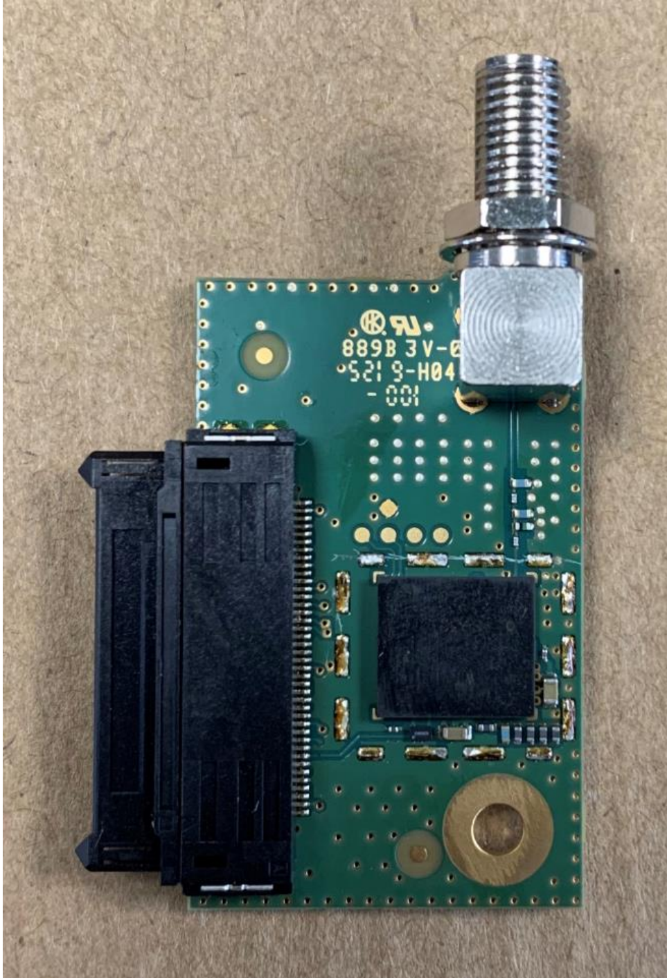
Figure 11. SCG2229 / XX6SCG2229 / 8739A-SCG2229 BT/Wi-Fi Board Top (Can Removed)
