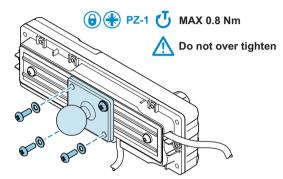
Fit a compatible mounting kit to the ball mount, such as a double socket arm. Ensure any mounting components are fully tightened after adjustments.
