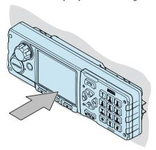
To remove, use the DIN release tools (provided)
