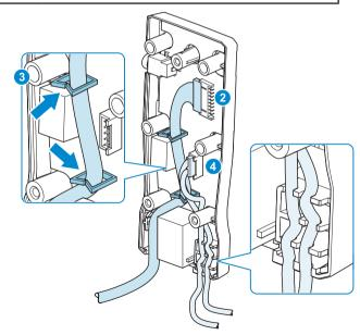
Screw the box halves back together securely, ensuring any cables are fitted correctly through the cable entry points. Plug the HBC3 into the interface box through the retaining clip and fold the clip back over the connector body to retain it securely in position.
