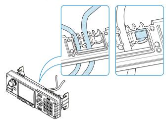
Fit the cable access cover over the cables and any bungs, using the screws provided.
