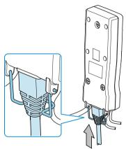
7. Fit the mounting bracket to the vehicle dash in a suitable location or directly to the interface box. Place the handset in the mounting bracket with the display facing the user.
