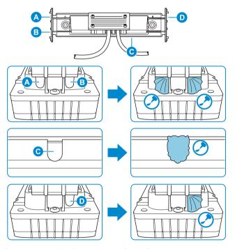
2. Place the assembly face-down on a flat surface until the sealant is dry.
