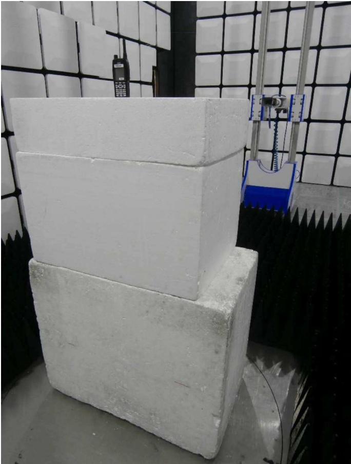
Figure 18 - Test Setup - 1 GHz to 18 GHz - Y Orientation
