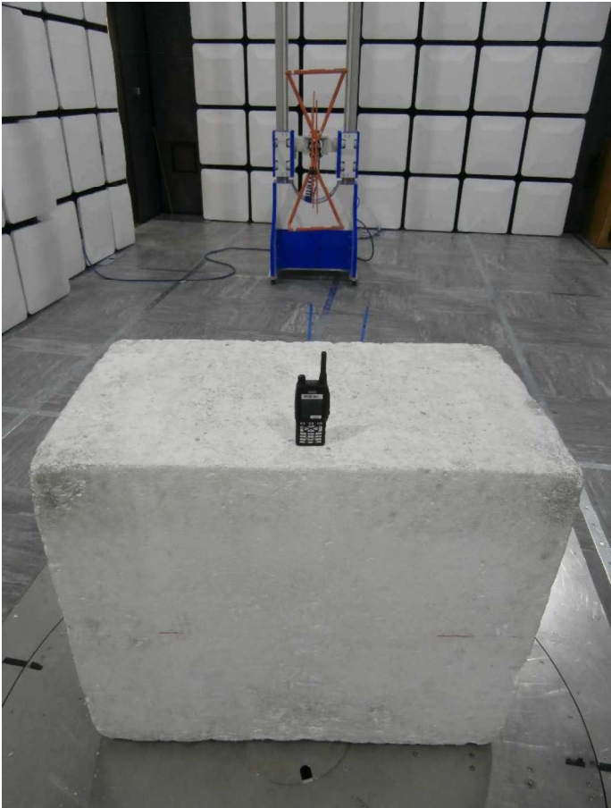
Figure 15 - Test Setup - 30 MHz to 1 GHz - Y Orientation
