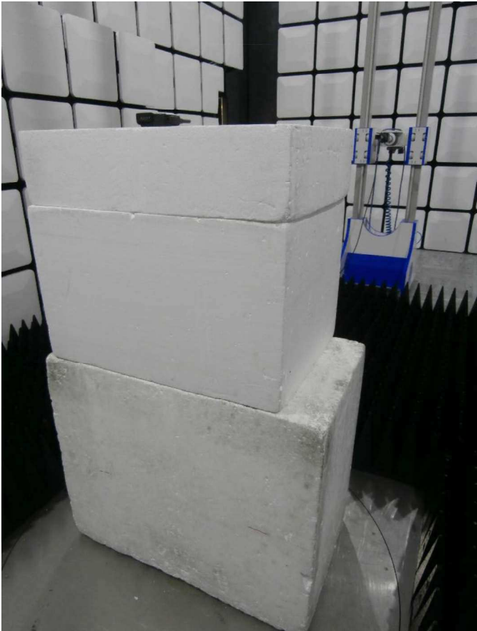
Figure 20 - Test Setup - 18 GHz to 25 GHz - X Orientation
