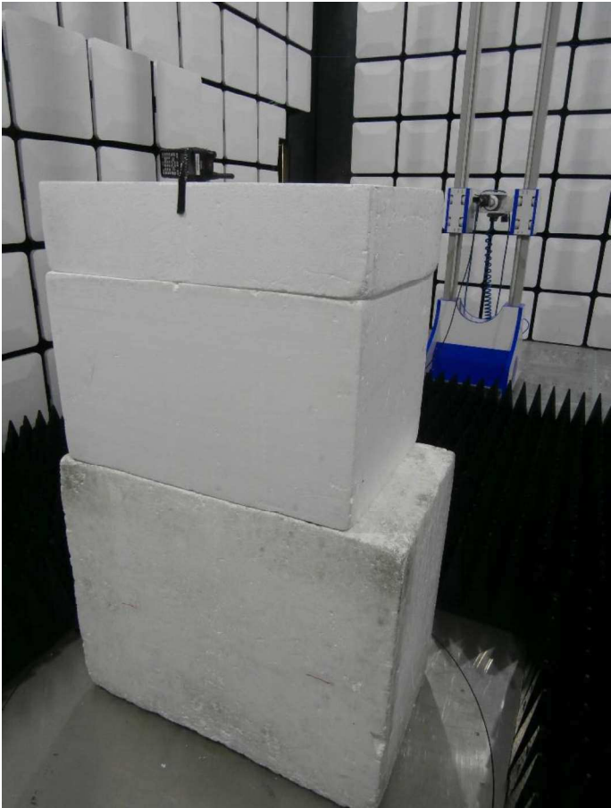
Figure 22 - Test Setup - 18 GHz to 25 GHz - Z Orientation
