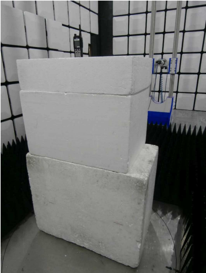
Figure 21 - Test Setup - 18 GHz to 25 GHz - Y Orientation
