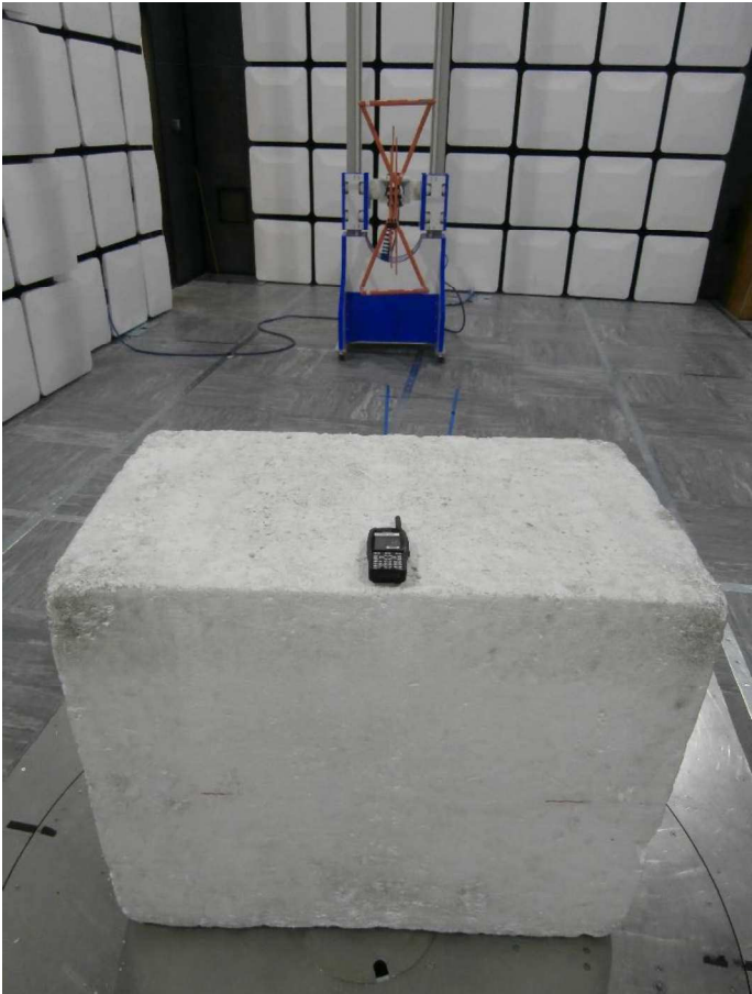
Figure 14 - Test Setup - 30 MHz to 1 GHz - X Orientation
