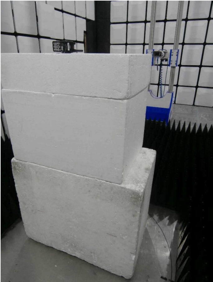
Figure 19 - Test Setup - 1 GHz to 18 GHz - Z Orientation
