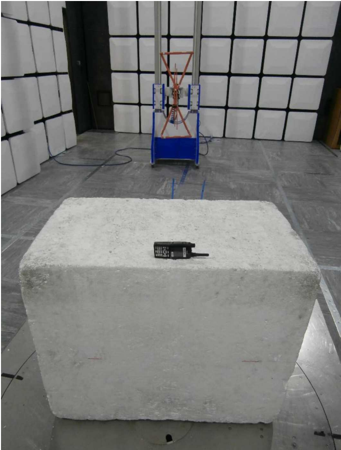
Figure 16 - Test Setup - 30 MHz to 1 GHz - Z Orientation
