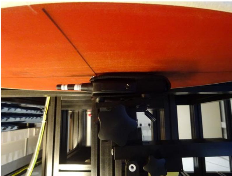
Figure 14: Rear face 1160 mAh Battery Fitted (Nylon Holster Fitted) – 0mm Separation Distance.
