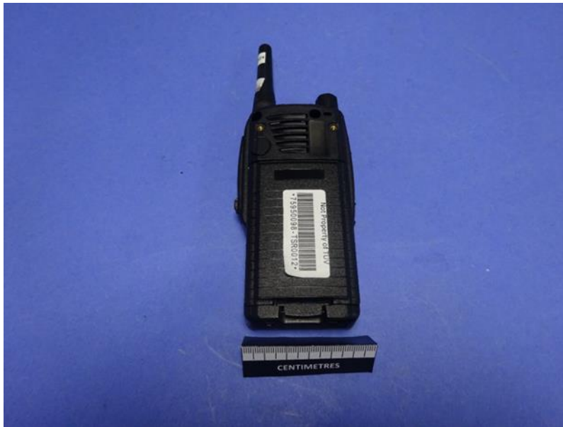
Figure 29: Rear – 1160 mAh Battery Fitted.
