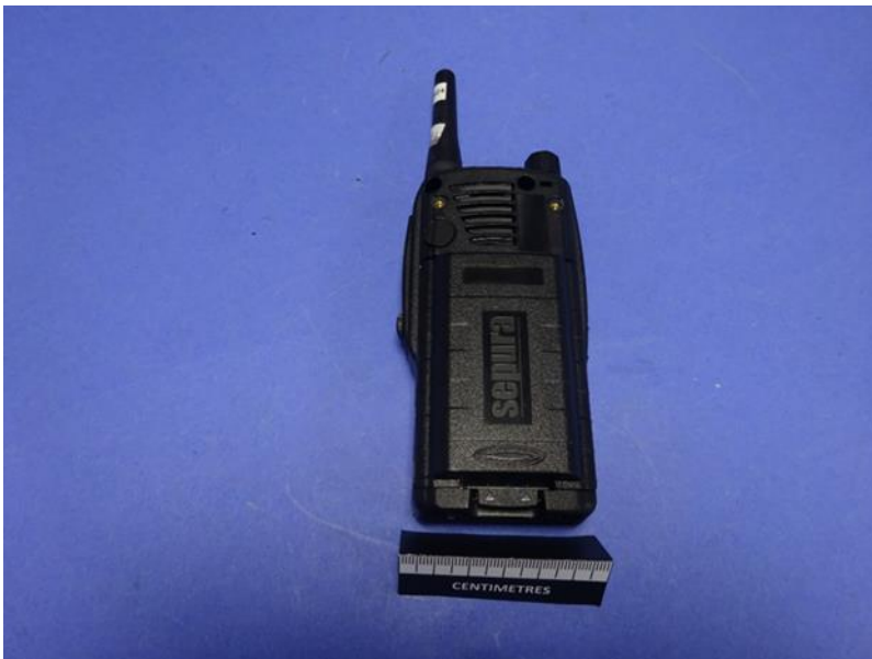
Figure 28: Rear – 1880 mAh Battery Fitted.
