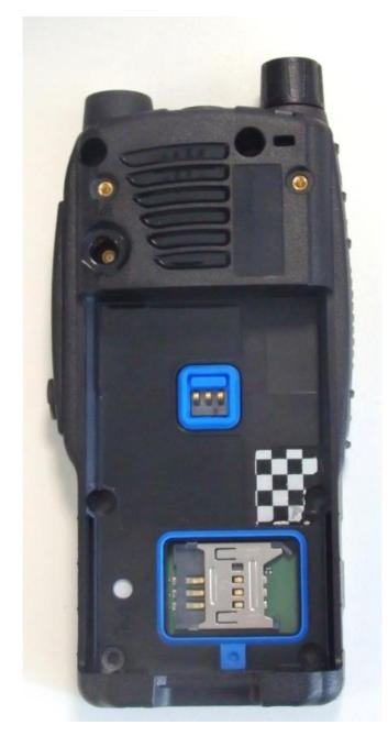
Figure 3. SC21 Series Rear with Battery and Antenna Removed
