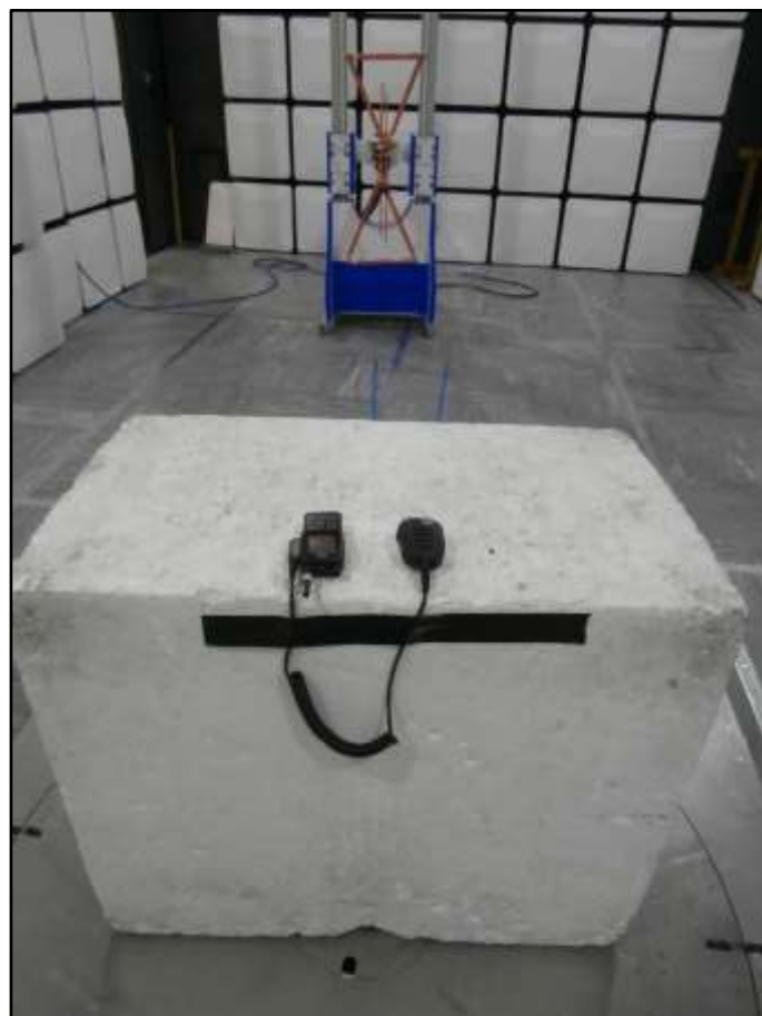
Figure 14 - Test Setup, 30 MHz to 1 GHz, X Orientation
