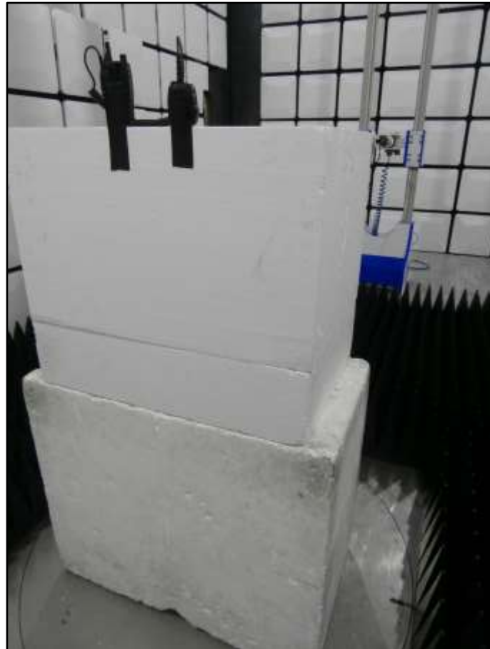
Figure 21 - Test Setup, 18 GHz to 25 GHz, Y Orientation
