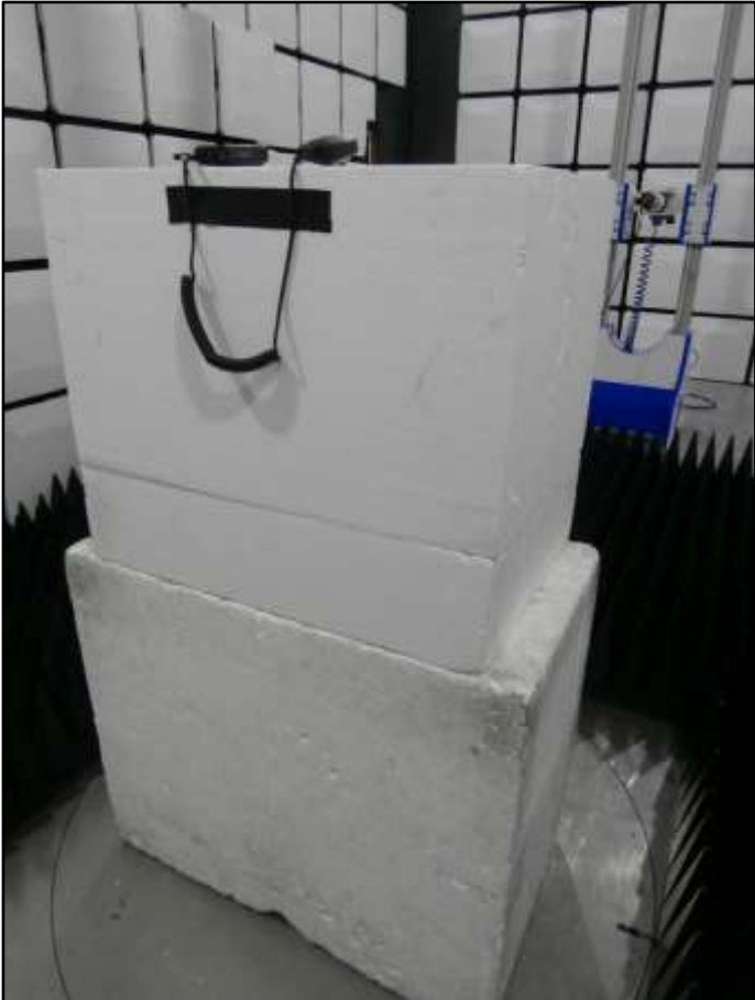
Figure 20 - Test Setup, 18 GHz to 25 GHz, X Orientation
