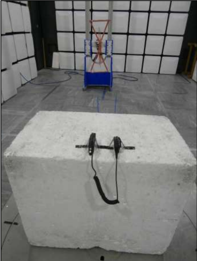
Figure 16 - Test Setup, 30 MHz to 1 GHz, Z Orientation
