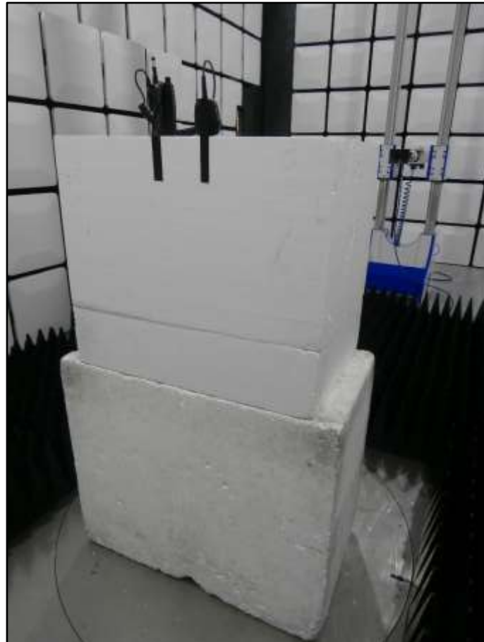
Figure 18 - Test Setup, 1 GHz to 18 GHz, Y Orientation
