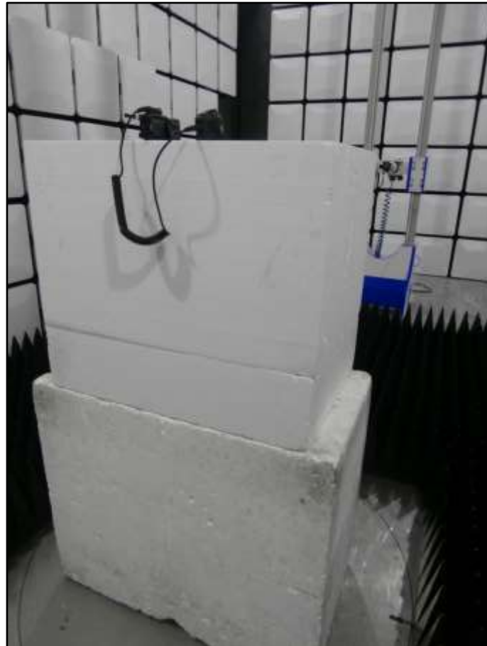
Figure 22 - Test Setup, 18 GHz to 25 GHz, Z Orientation
