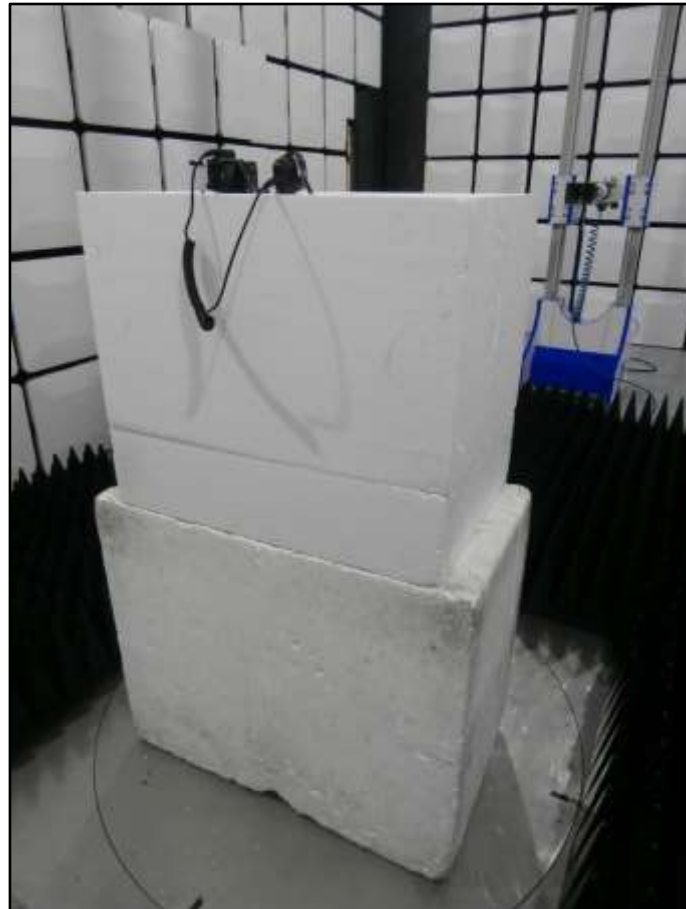
Figure 19 - Test Setup, 1 GHz to 18 GHz, Z Orientation
