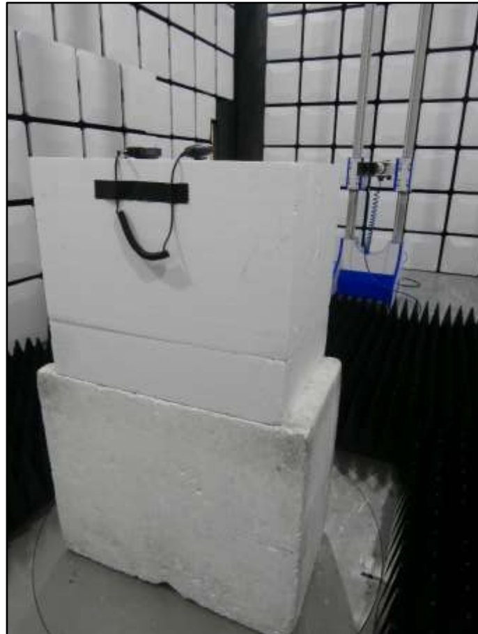
Figure 17 - Test Setup, 1 GHz to 18 GHz, X Orientation
