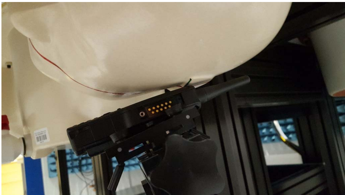
SAR - Head - Left 15° - 1880 mAh Battery
