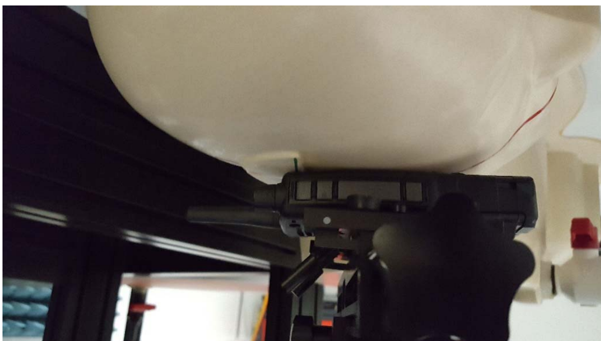
SAR - Head - Right Cheek - 1880 mAh Battery
