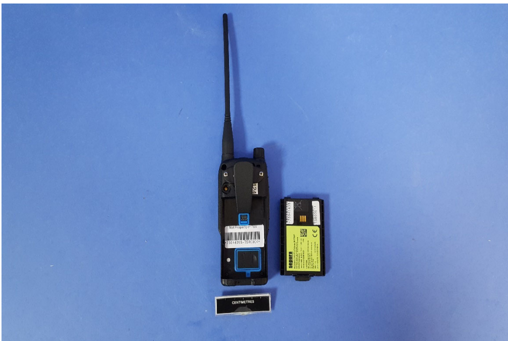
Figure 106 Rear (1/4 Wave Whip Antenna - part no: 310-00015 fitted ), 1160 mAh Battery (Part no: 300-01852) - Open
