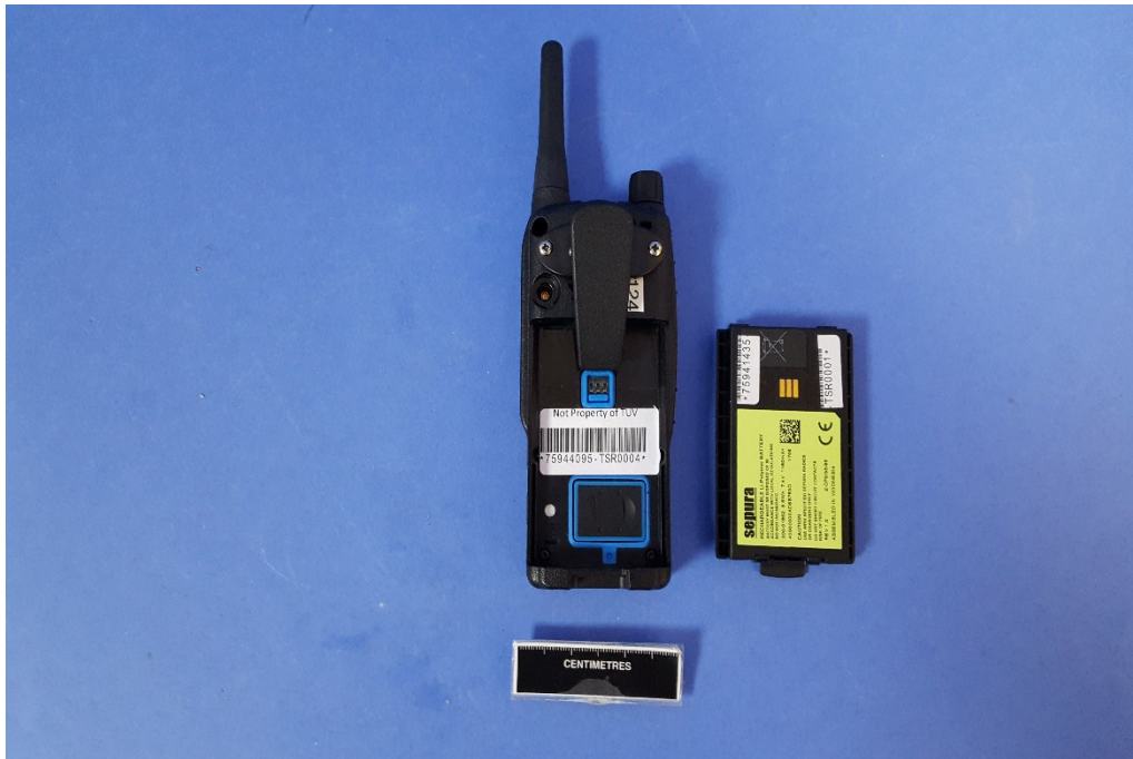
Figure 101 Rear (Extended helical antenna part no:300-01931 fitted ), 1160 mAh Battery (Part no: 300-01852) - Open Note: Extended helical antenna - part no:300-01960 has identical dimensions
