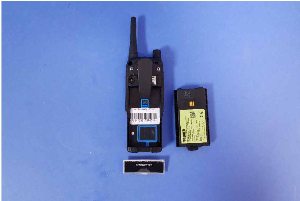
Figure 103 Rear (Extended helical antenna part no:300-01931 fitted ), 1880 mAh Battery (Part no: 300-01853) - Open Note: Extended helical antenna - part no:300-01960 has identical dimensions
