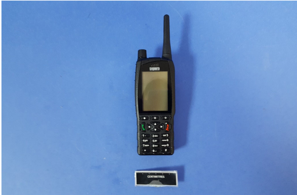
Figure 99 Front (Extended helical antenna part no:300-01931 fitted ) Note: Extended helical antenna part no:300-01960 has identical dimensions
