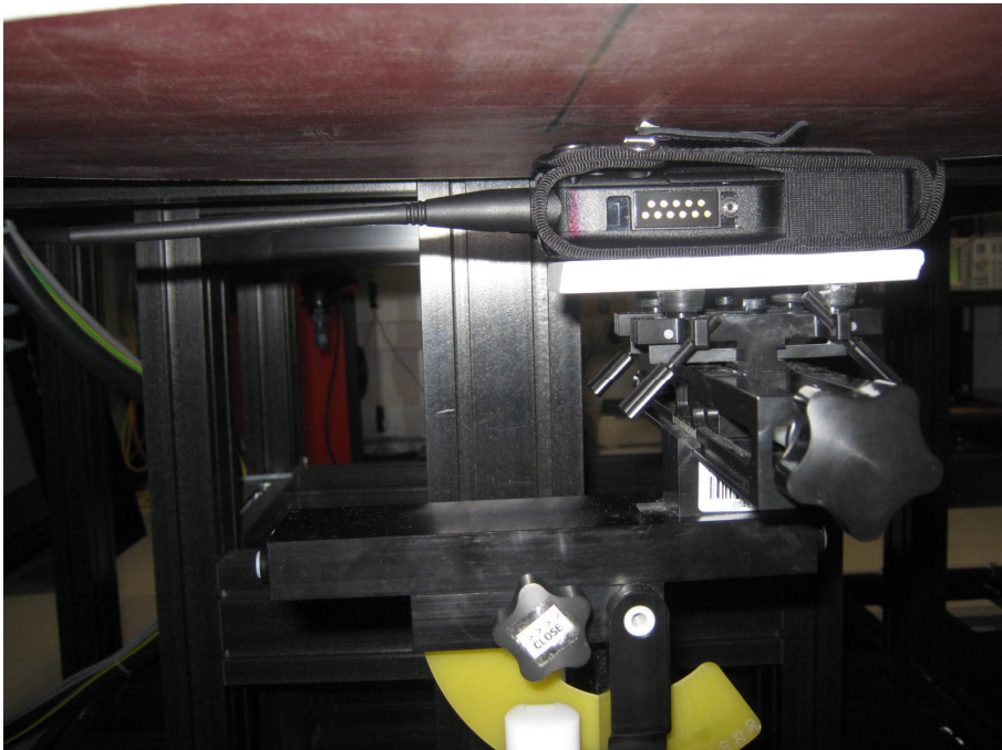
Figure 65 Rear Face - 1160 mAh Battery (Part no: 300-01852) Whip Antenna (Part no: 310-00015) Holster 300-01915 (Leather) 0 mm Separation distance
