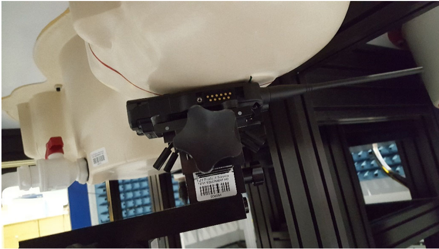
Figure 94 Left Cheek - 1880 mAh Battery (Part no: 300-01853) ¼ Wave Whip Antenna (Part no: 310-00015)
