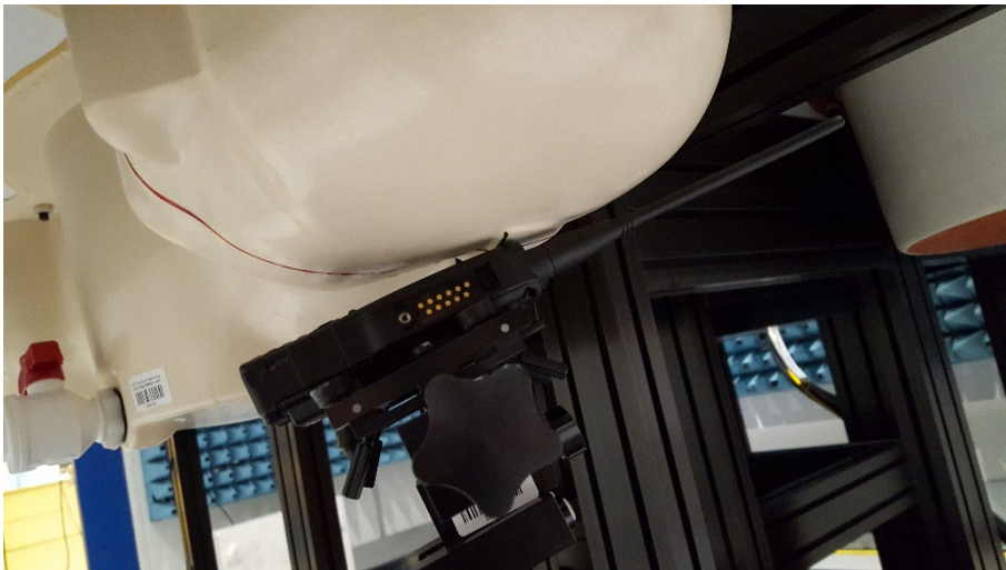
Figure 93 Left Tilt - 1880 mAh Battery (Part no: 300-01853) ¼ Wave Whip Antenna (Part no: 310-00015)
