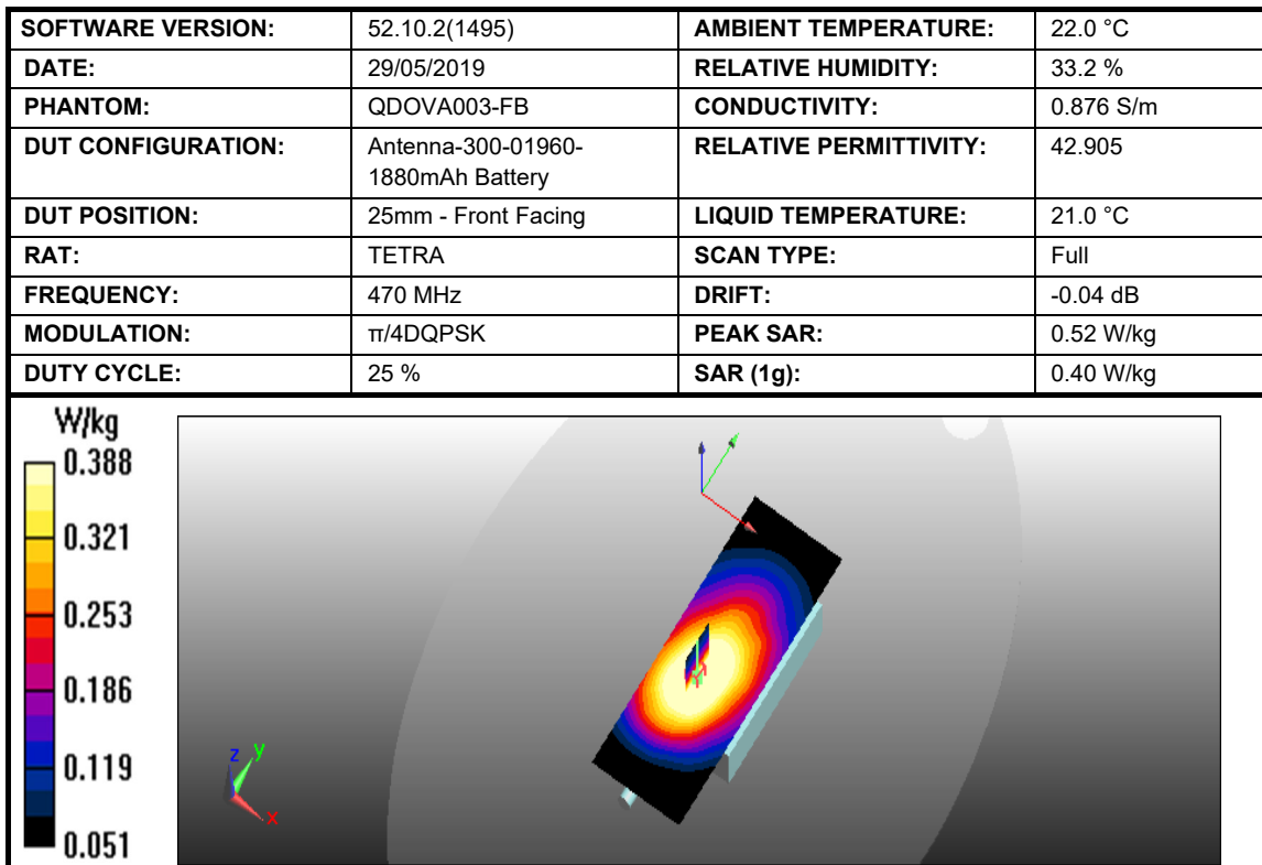
Figure 6: SAR Front Of Face Testing Results for the SC2124 at 470 MHz.
