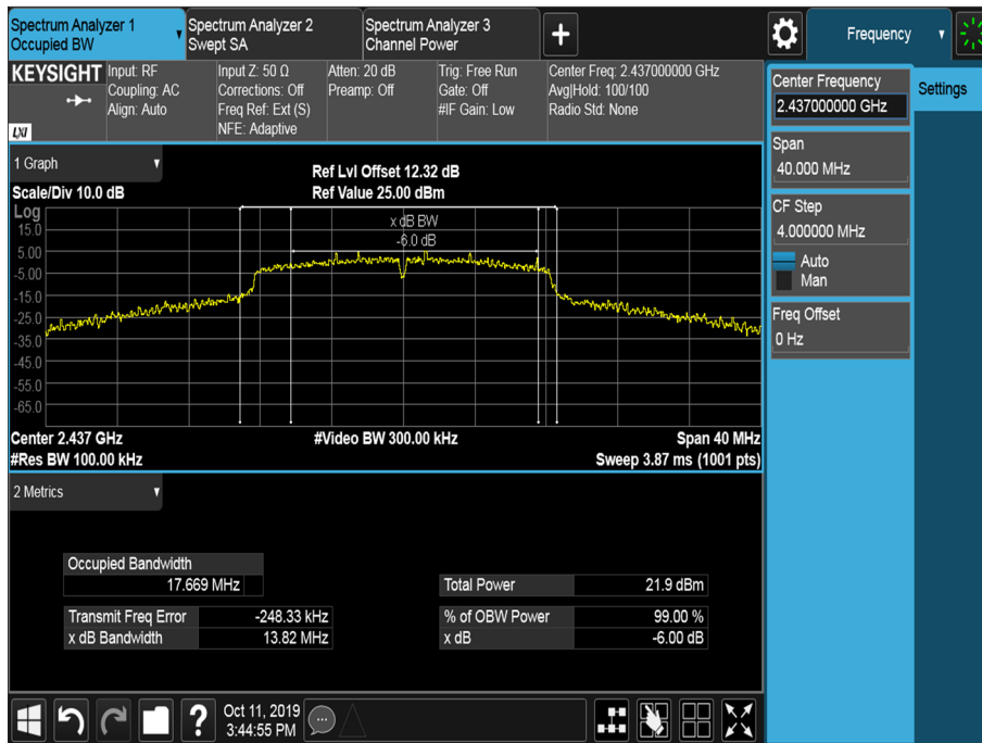
Figure 5 - 2437 MHz – 6 dB Bandwidth and 99 % Occupied Bandwidth
