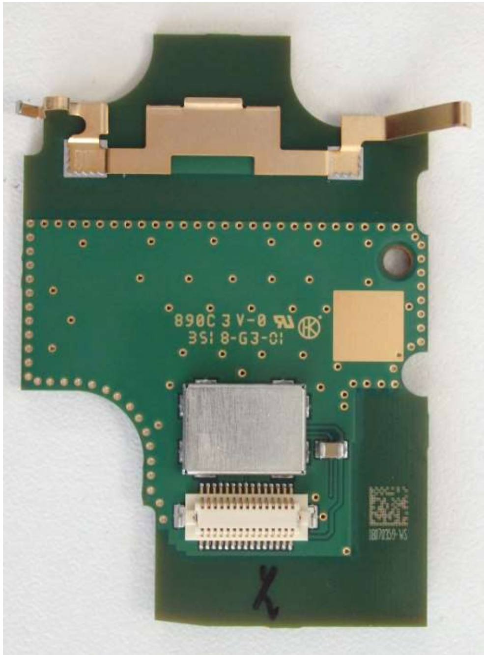
Figure 5. XX6SC2124 GPS Module Rear View
