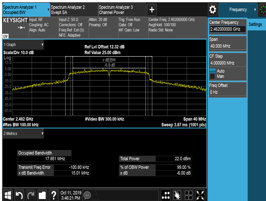
Figure 6 - 2462 MHz – 6 dB Bandwidth and 99 % Occupied Bandwidth
