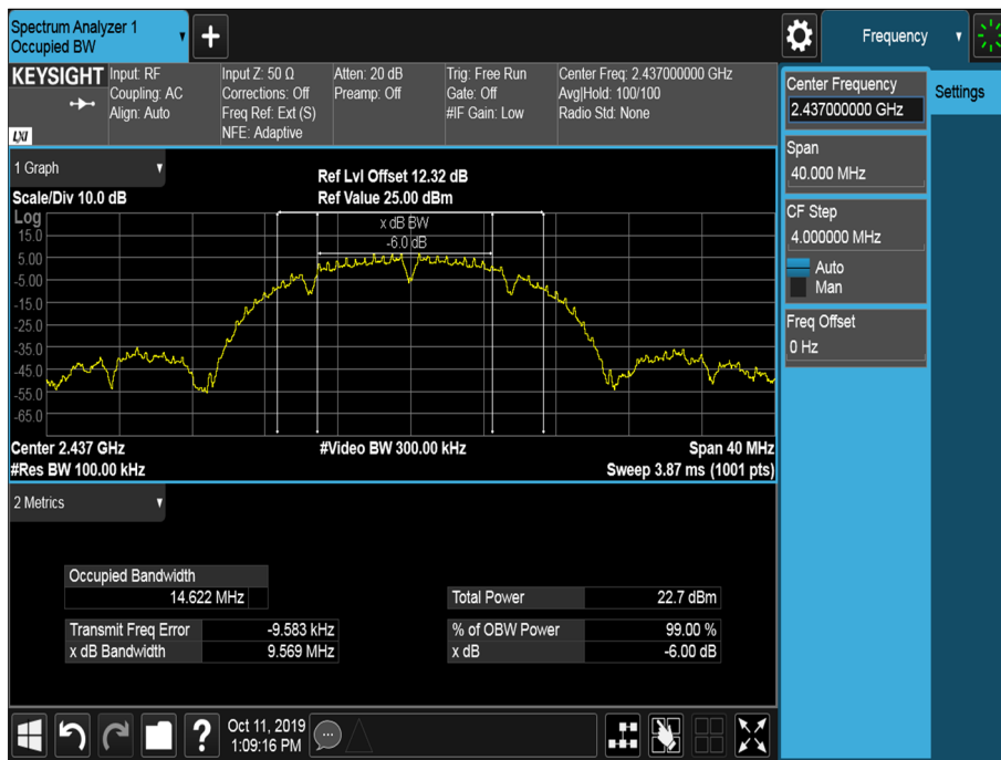
Figure 2 - 2437 MHz – 6 dB Bandwidth and 99 % Occupied Bandwidth
