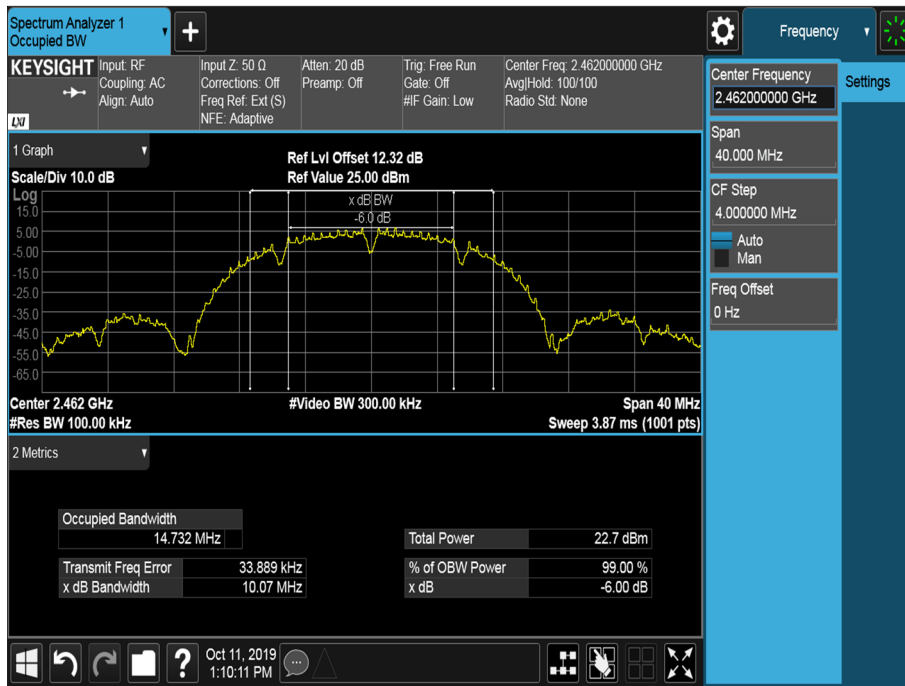
Figure 3 - 2462 MHz – 6 dB Bandwidth and 99 % Occupied Bandwidth
