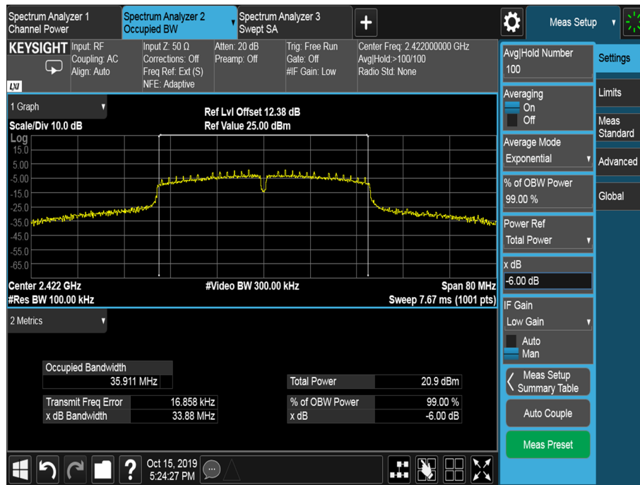
Figure 10 - 2422 MHz 6 dB Bandwidth and 99 % Occupied Bandwidth
