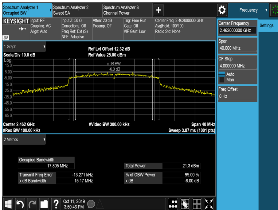
Figure 9 - 2462 MHz 6 dB Bandwidth and 99 % Occupied Bandwidth
