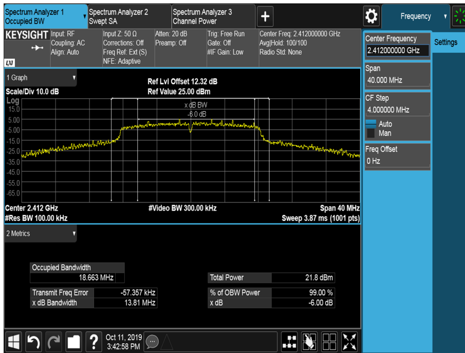
Figure 4 - 2412 MHz – 6 dB Bandwidth and 99 % Occupied Bandwidth
