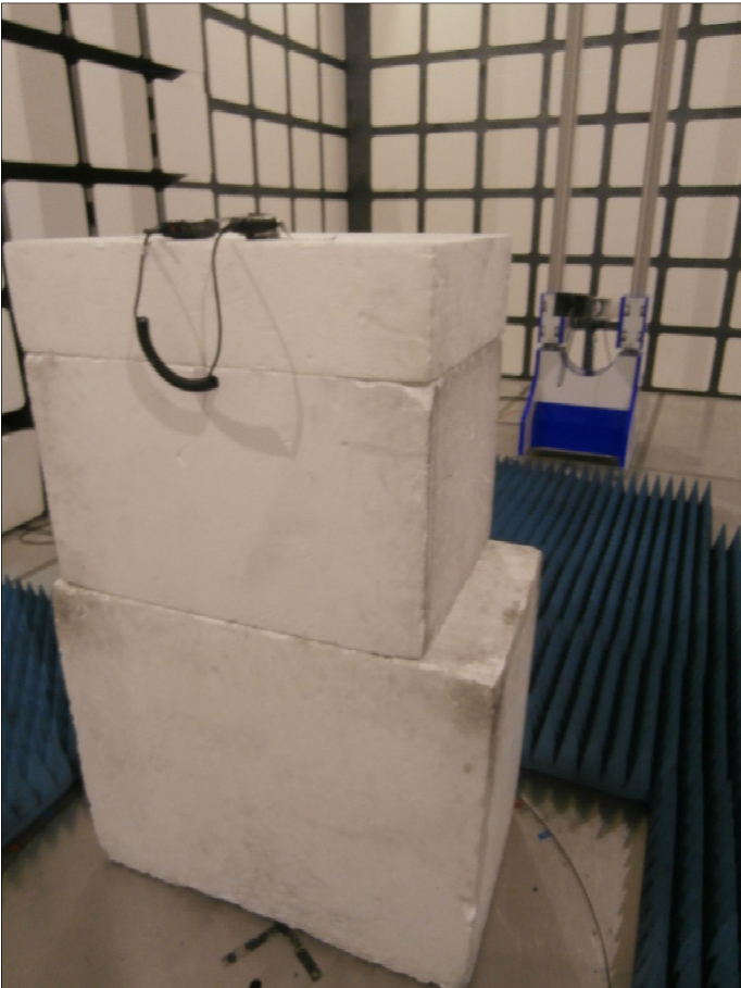
Figure 147 - Test Setup – 1 GHz to 18 GHz
