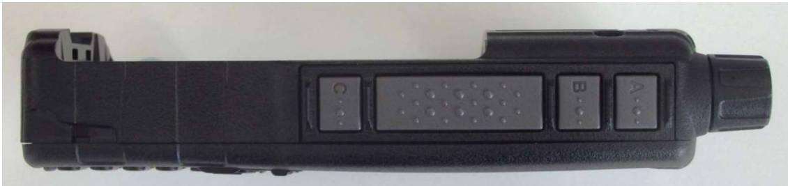
Figure 6. XX6SC2124 PTT Side with Battery and Antenna Removed
