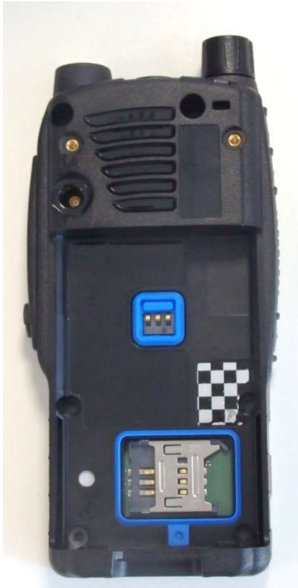
Figure 3. XX6SC2124 Rear with Battery and Antenna Removed
