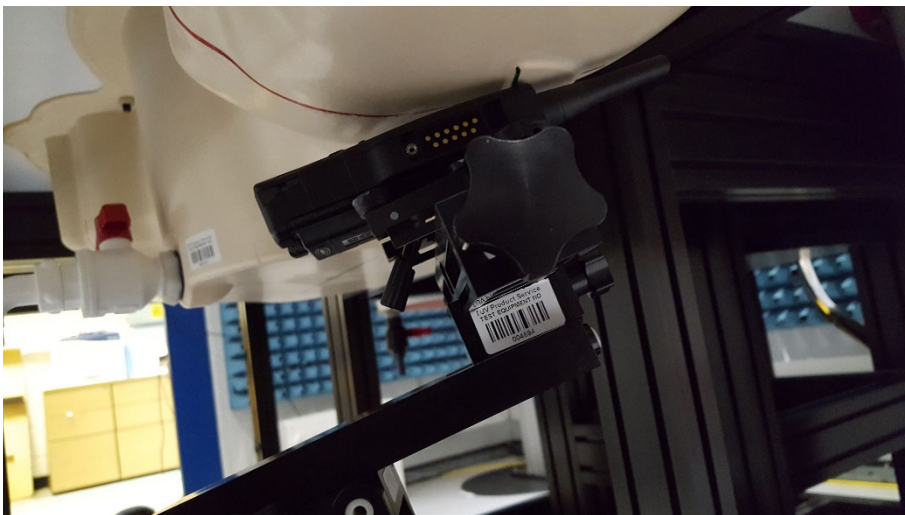
Figure 85 Left Tilt - 1880 mAh Battery (Part no: 300-01853) Extended Helical Antenna (Part no: 300-01931)
