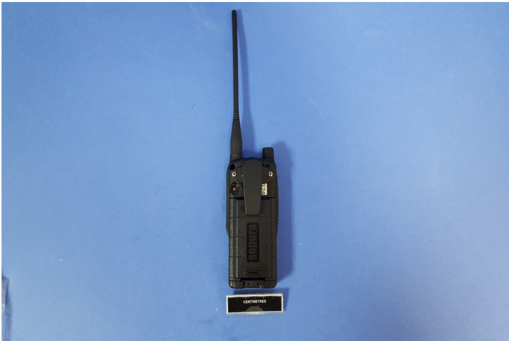
Figure 107 Rear (1/4 Wave Whip Antenna - part no: 310-00015 fitted ), 1880 mAh Battery (Part no: 300-01853)
