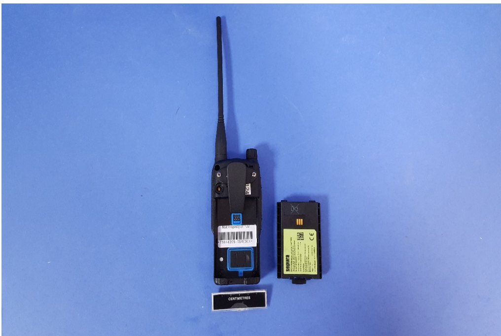
Figure 108 Rear (1/4 Wave Whip Antenna - part no: 310-00015 fitted ), 1880 mAh Battery (Part no: 300-01853) - Open
