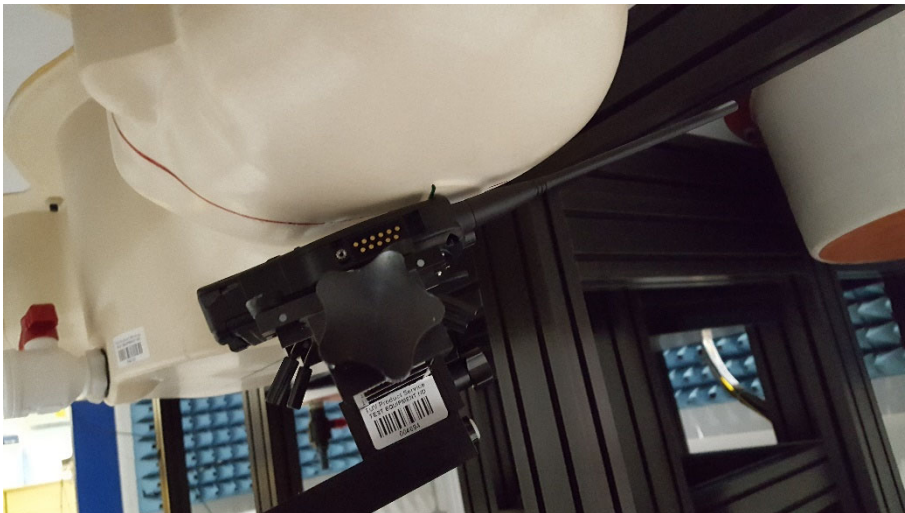
Figure 97 Left Tilt - 1160 mAh Battery (Part no: 300-01852) ¼ Wave Whip Antenna (Part no: 310-00015)
