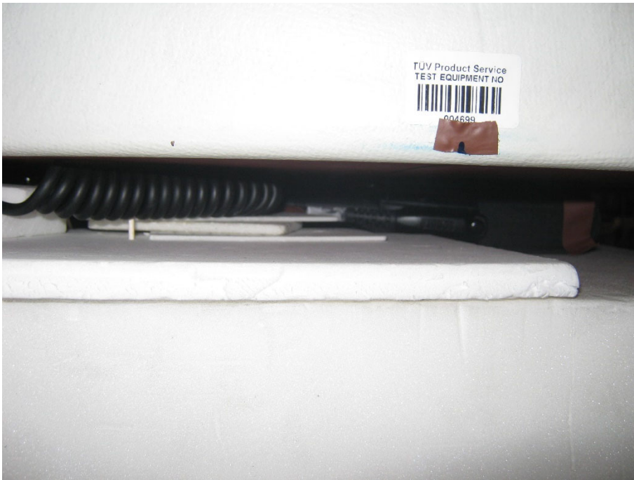
Figure 74 Rear Face - 1160 mAh Battery (Part no: 300-01852) Whip Antenna (Part no: 310-00015) Holster 300-01916 (Nylon) RSM attached 0 mm Separation distance
