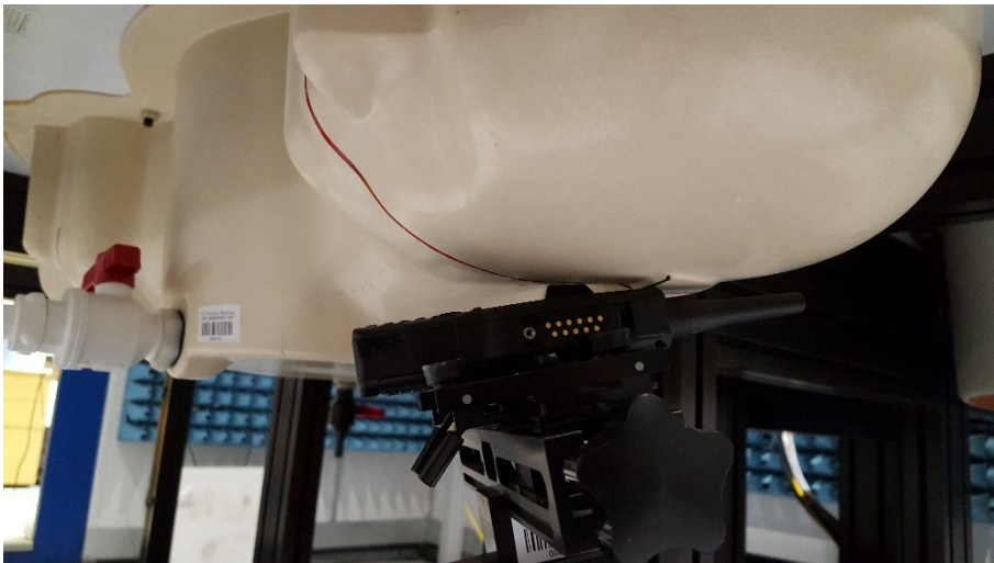
Figure 89 Left Tilt - 1160 mAh Battery (Part no: 300-01852) Extended Helical Antenna (Part no: 300-01931)
