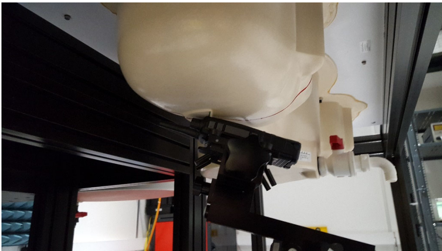
Figure 87 Right Tilt - 1160 mAh Battery (Part no: 300-01852) Extended Helical Antenna (Part no: 300-01931)
