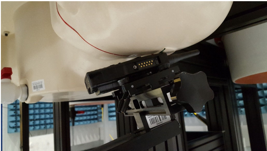
Figure 77 Left Tilt - 1880 mAh Battery (Part no: 300-01853) Extended Helical Antenna (Part no: 300-01960)
