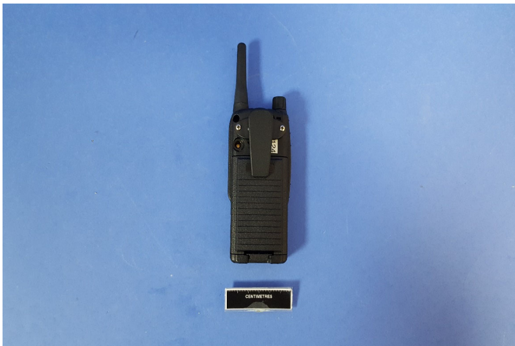
Figure 100 Rear (Extended helical antenna part no:300-01931 fitted ), 1160 mAh Battery (Part no: 300-01852) Note: Extended helical antenna - part no:300-01960 has identical dimensions
