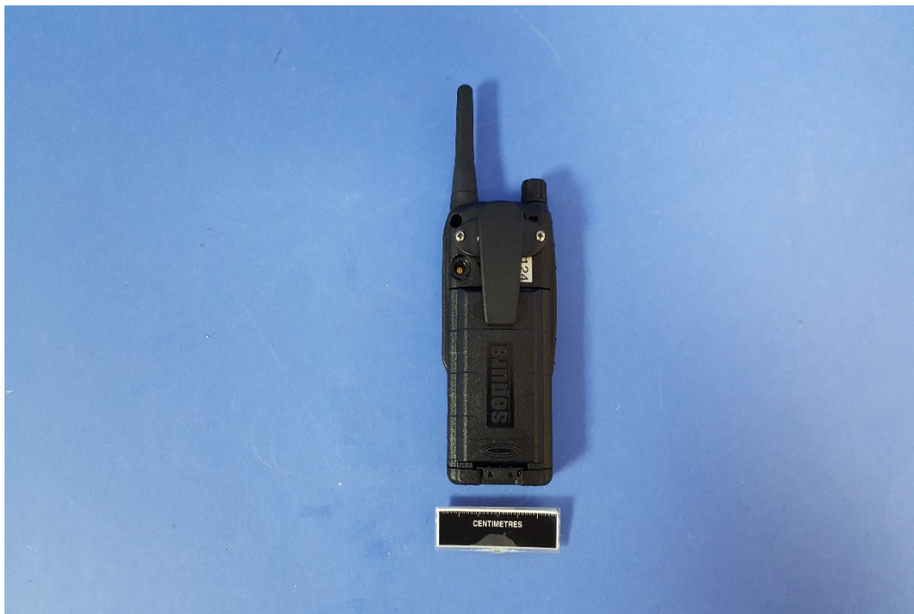
Figure 102 Rear (Extended helical antenna part no:300-01931 fitted ), 1880 mAh Battery (Part no: 300-01853) Note: Extended helical antenna - part no:300-01960 has identical dimensions
