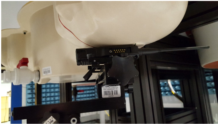
Figure 98 Left Cheek - 1160 mAh Battery (Part no: 300-01852) ¼ Wave Whip Antenna (Part no: 310-00015)
