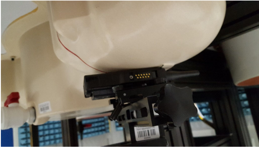
Figure 78 Left Cheek - 1880 mAh Battery (Part no: 300-01853) Extended Helical Antenna (Part no: 300-01960)
