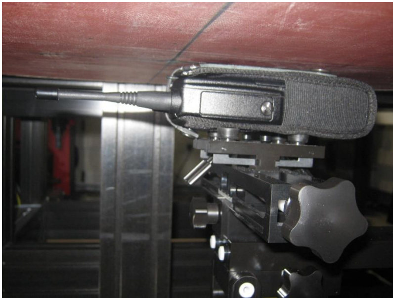
Figure 46 Rear face - 1160 mAh battery with Nylon Holster and belt clip
