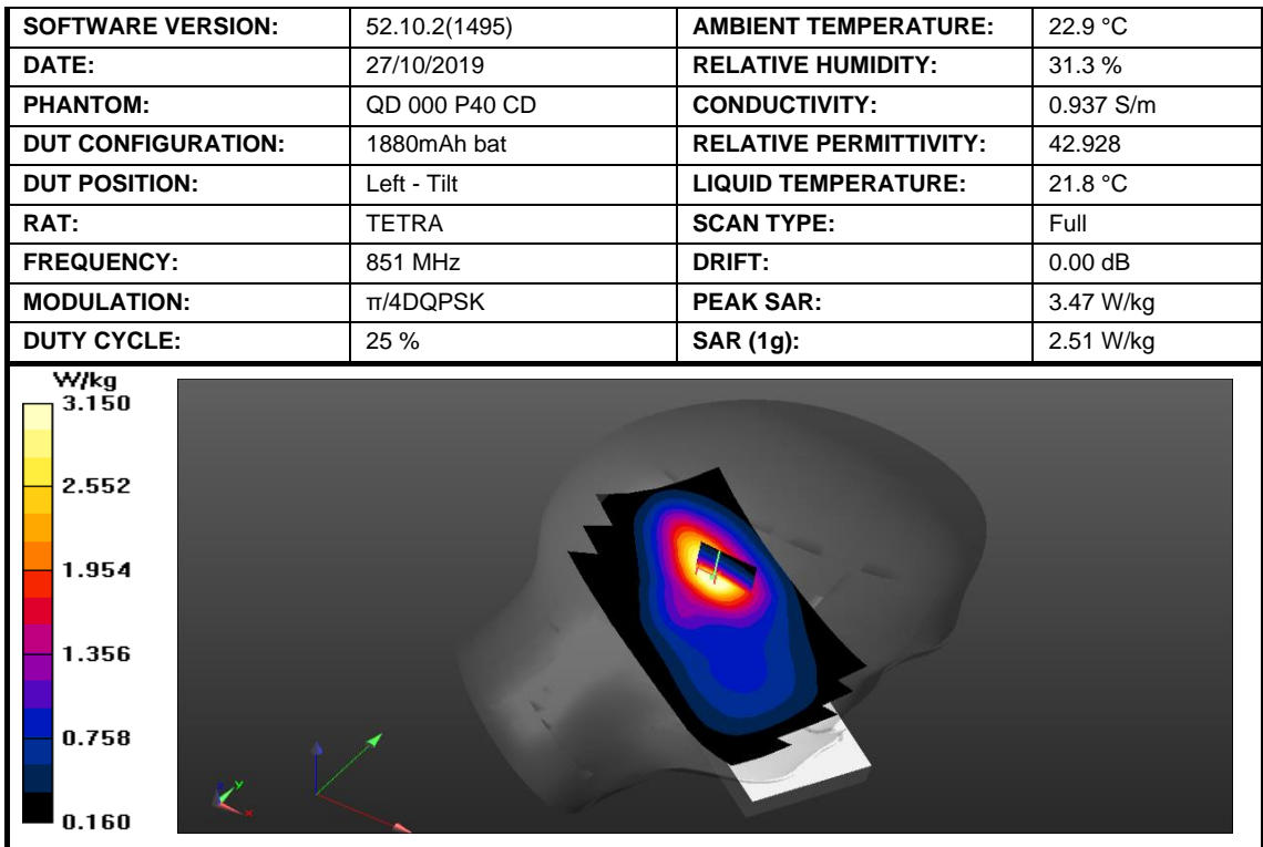
Figure 11: SAR Head Testing Results for the SC2028 at 851 MHz.
