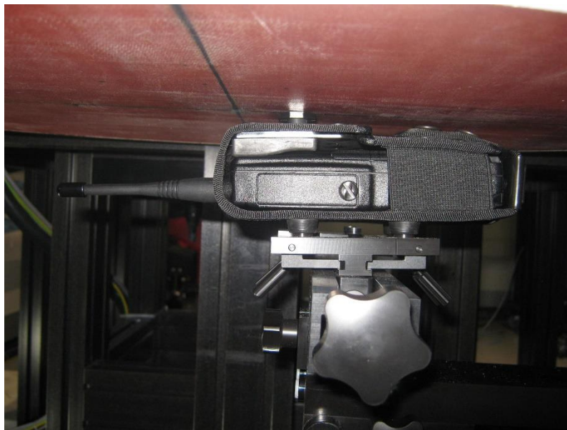
Figure 45 Rear face - 1160 mAh battery with Leather click fast holster
