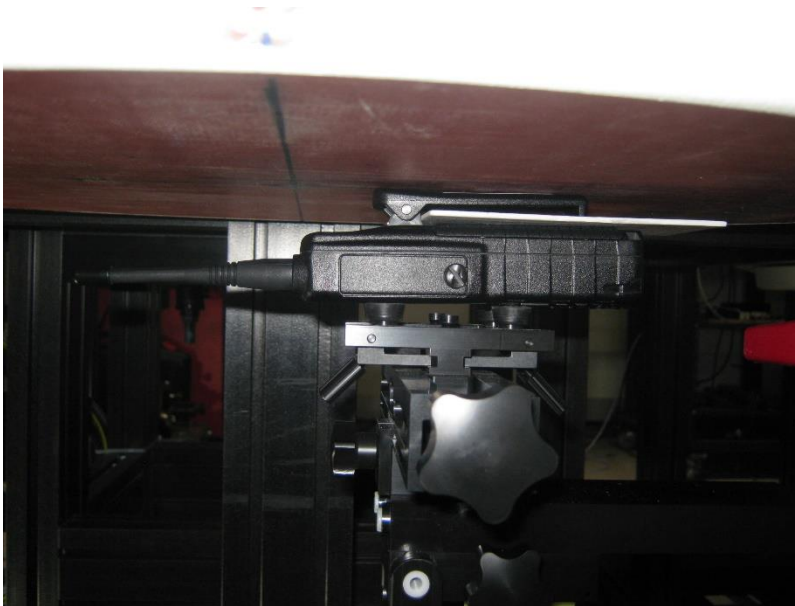
Figure 43 Rear face - 1160 mAh battery with large clip
