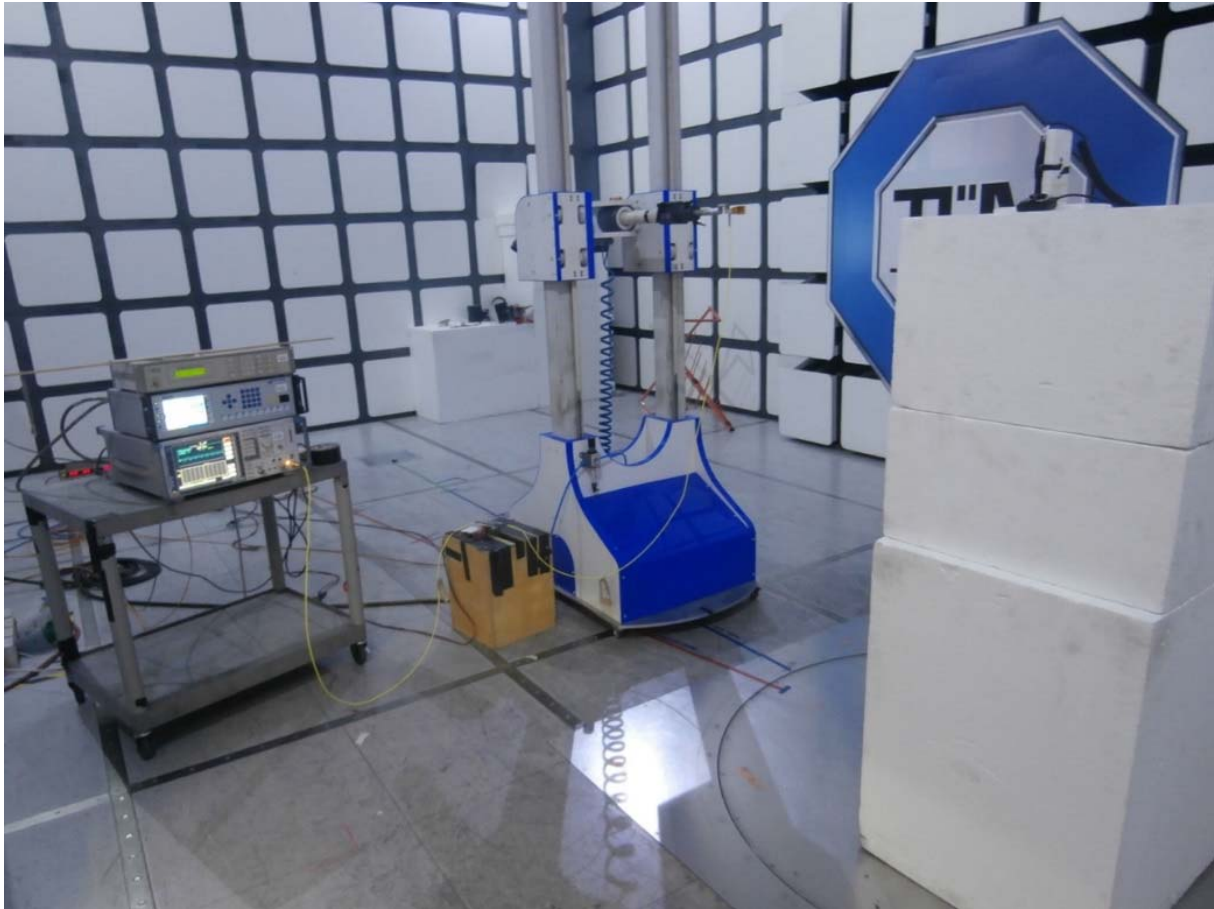
FCC Part 15.407 Radiated Emissions 18 GHz to 25 GHz
