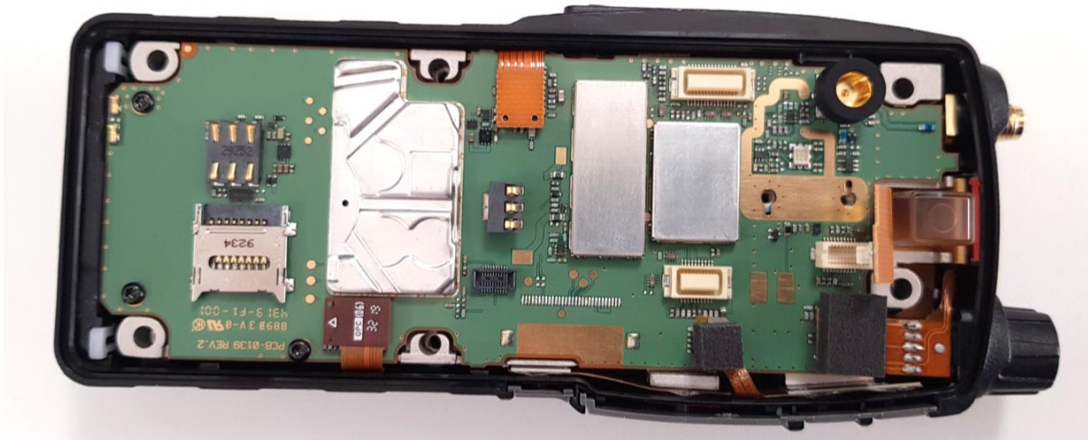
Figure 4. SC2028 Main PCB with Heatsink Removed
