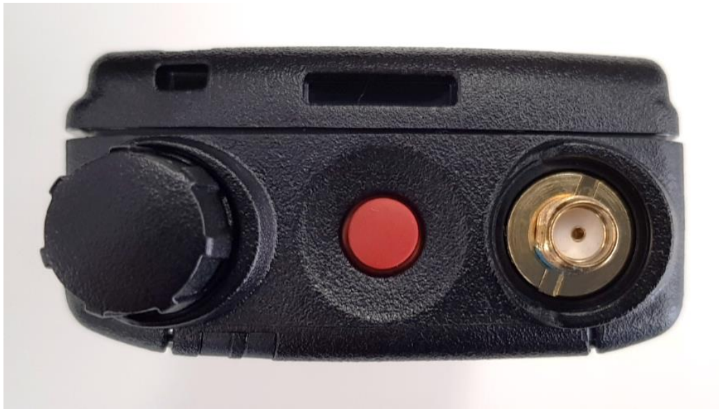
Figure 4. XX6SC2028 Top with Battery and Antenna Removed
