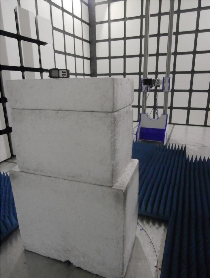
Figure 98 – Radiated Emission Setup, EUT Orientation Y
