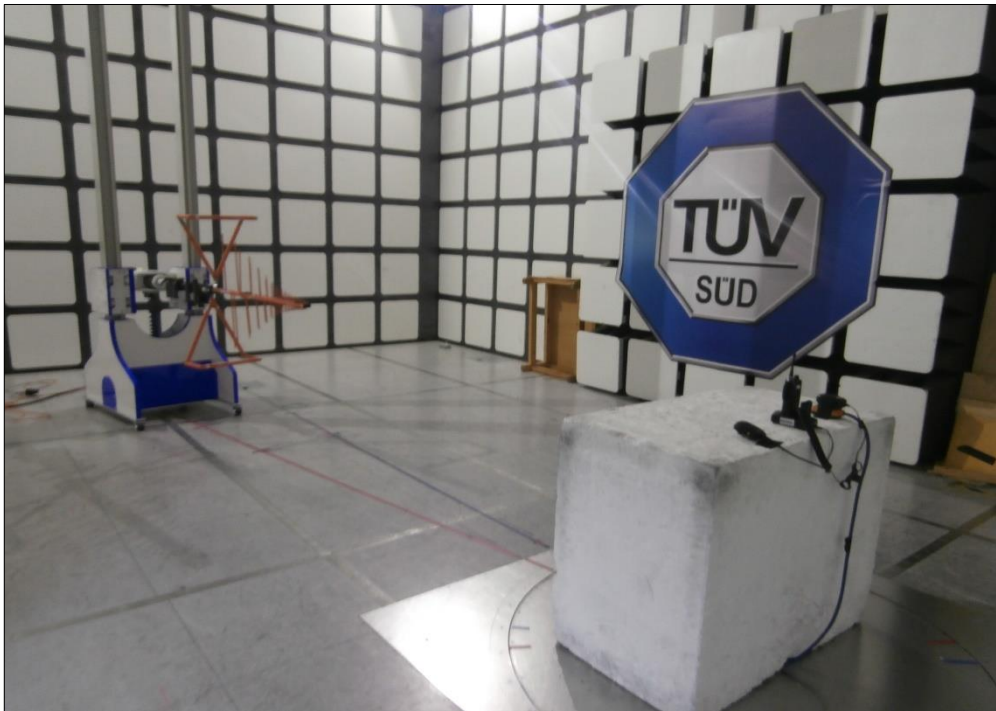
Figure 23 - Test Setup - 30 MHz to 1 GHz
