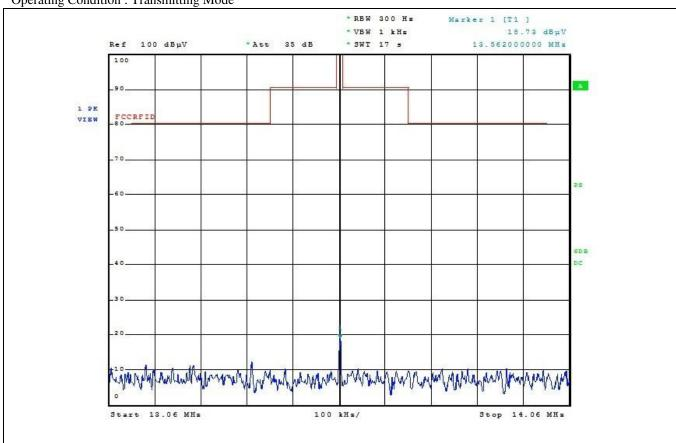
cc. to above test data, the field strength level of 13.558 7 MHz is 56.98 dBuV/m and the worst limit subject to 15.225 (b) and (c) is 80.5 dBuV/m, so the EUT meets the requirement.
