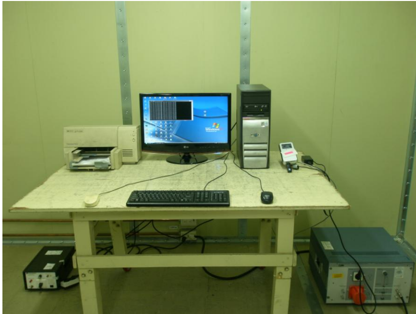
Photograph 3 : Setup for Conducted Emissions
