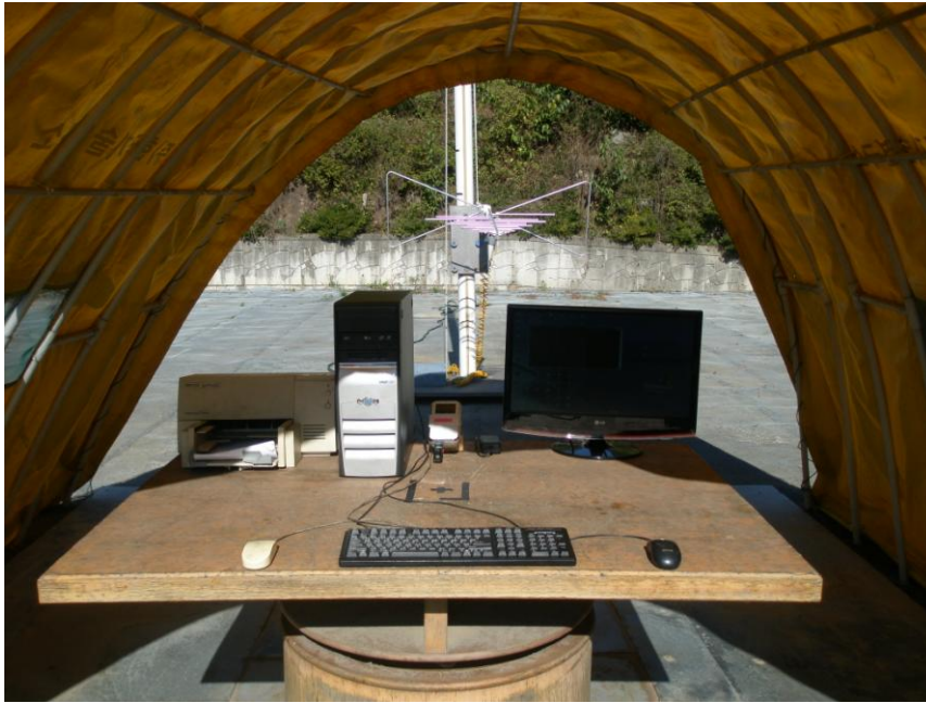
Photograph 2 : Setup for radiated Emissions (above 30 MHz)
