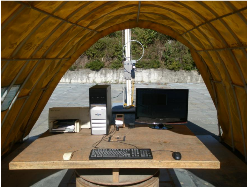
Photograph 1 : Setup for radiated Emissions (below 30 MHz)
