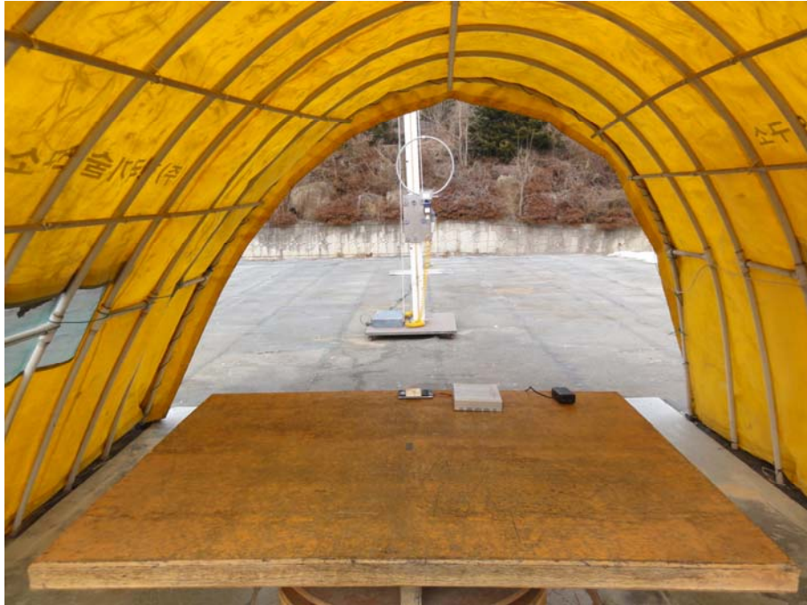
Photograph 1 : Setup for radiated Emissions (below 30 MHz)
