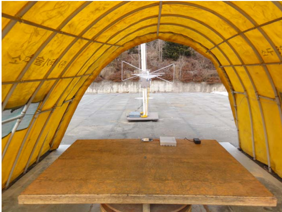
Photograph 2 : Setup for radiated Emissions (above 30 MHz)
