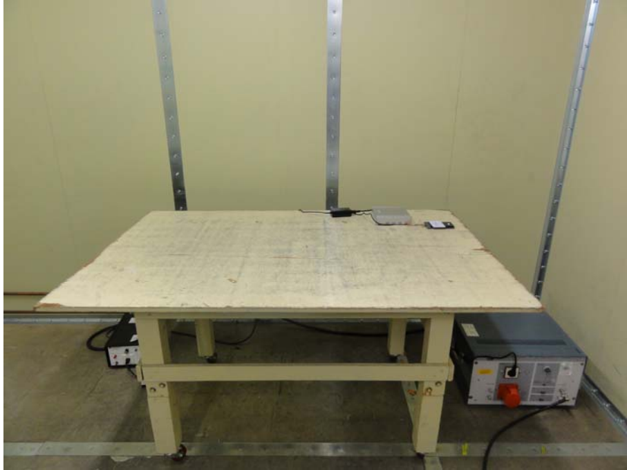
Photograph 3 : Setup for Conducted Emissions
