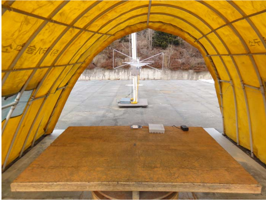
Photograph 2 : Setup for radiated Emissions (above 30 MHz)
