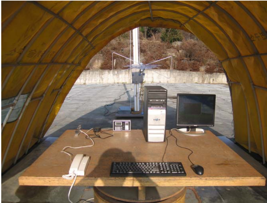
Photograph 2 : Setup for radiated Emissions (above 30 MHz)
