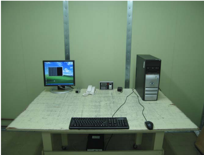
Photograph 3 : Setup for Conducted Emissions
