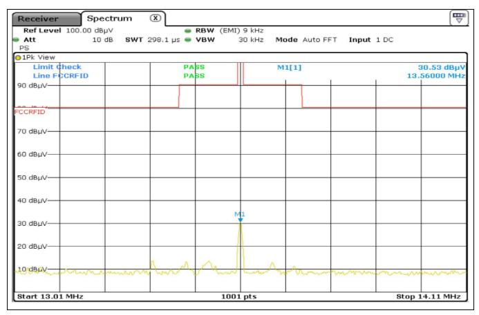
cc. to above test data, the field strength level of 13.56 MHz is 30.53 dBuV/m and the worst limit subject to 15.225 (b) and
