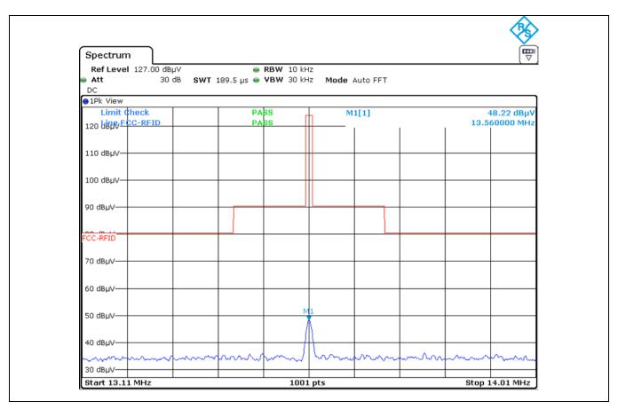
cc. to above test data, the field strength level of 13.56 MHz is 48.22 dBuV/m and the worst limit subject to 15.225 (b) and (c) is 80.5 dBuV/m, so the EUT meets the requirement.
