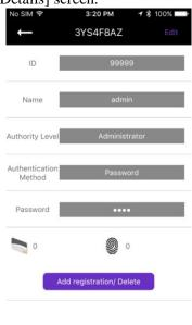
When you select the [Save] button after modifying the items except the ID, if there is any additional authentication means, the terminal becomes the input standby status and carries out additional registration.
