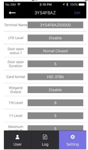
To change the terminal settings, press the [Edit] button on the top right to switch to the edit mode.
