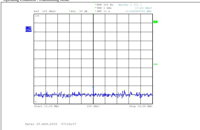
cc. to above test data, the field strength level of 13.560 4 MHz is 17.64 dBuV/m and the worst limit subject to 15.225 (b) and (c) is 80.5 dBuV/m, so the EUT meets the requirement.
